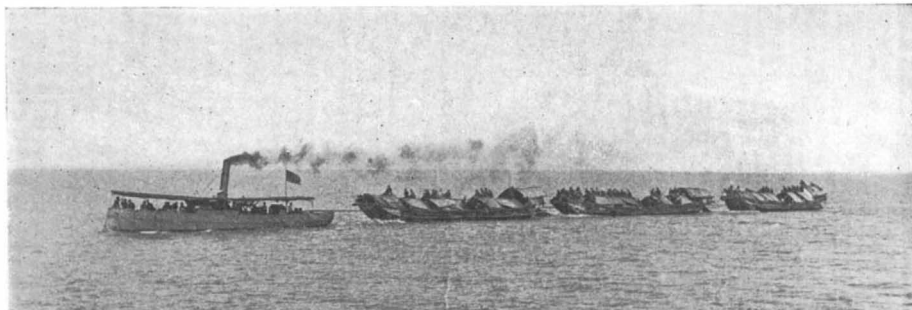
Launch Towing Loaded Cascoes from the Transports to the Docks at Manila.
