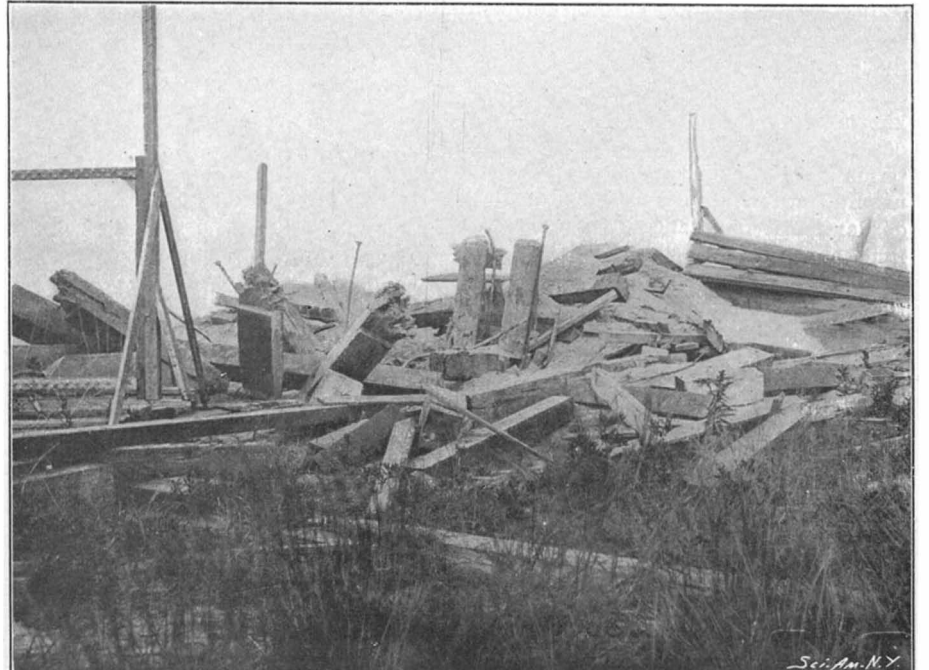
THE TARGET AFTER BEING STRUCK BY GATHMANN 12-INCH SHELL, CONTAINING 800 POUNDS OF WET GUNCOTTON.
