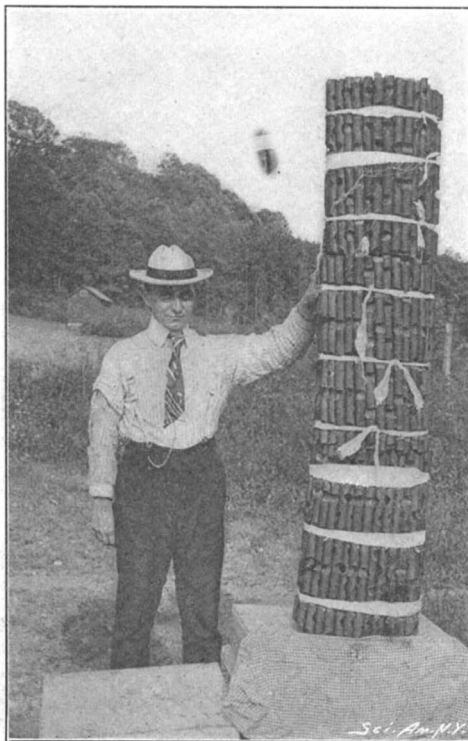
POWDER CHARGE FOR 12-INCH TORPEDO GUN.
