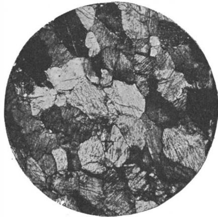
Micro-Photograph of Carrara Marble Before Compression.
