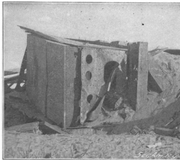
SIDE VIEW SHOWING CRUSHING EFFECT OF GATHMANN SHELL ON PLATE STEEL BACKING.
