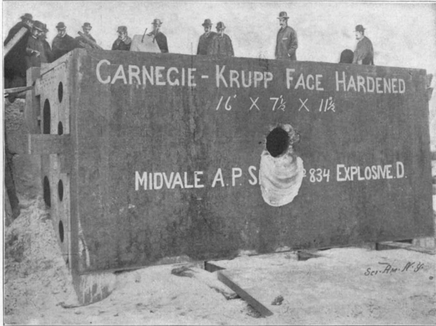
Armor-Piercing Shot Test. First Round. Plate Penetrated and Backing Wrecked.
