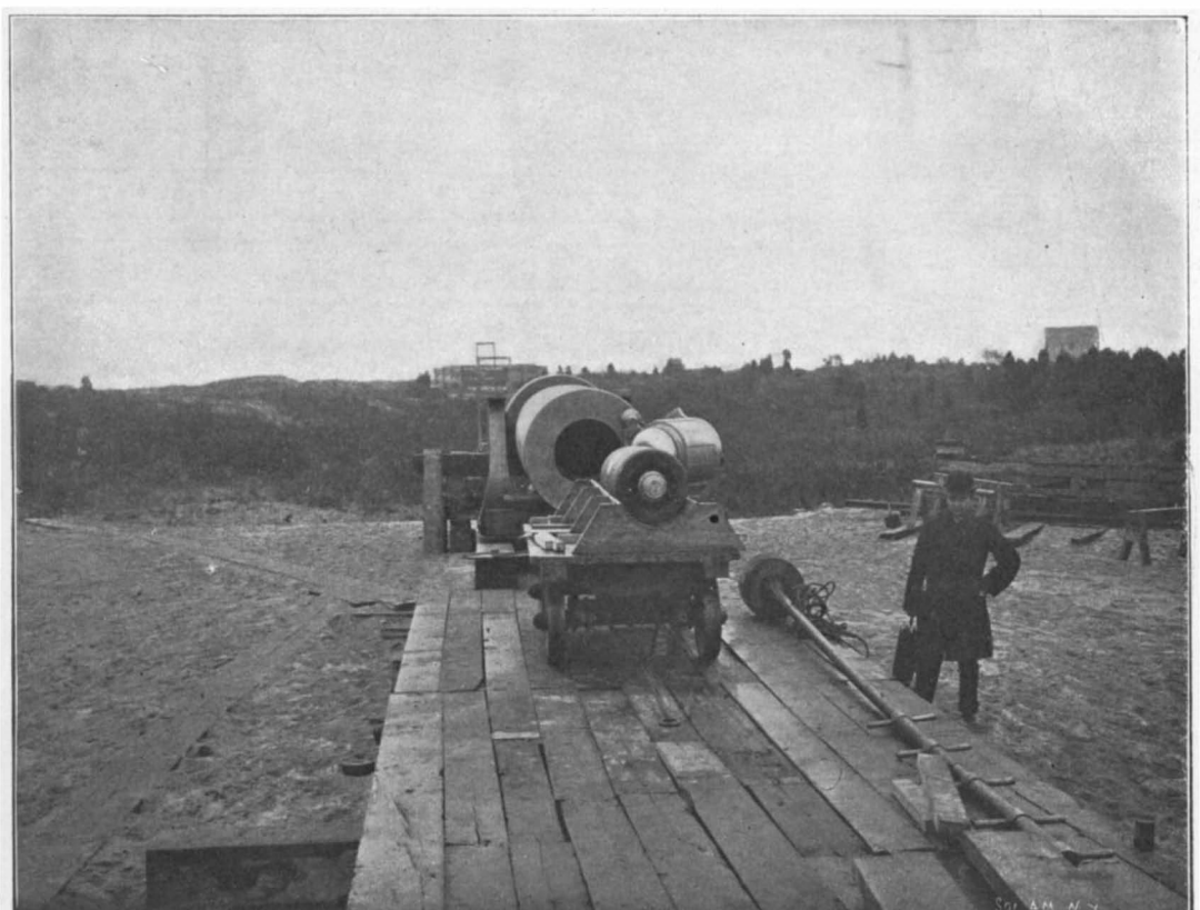
Gathmann Shell Test. View from Rear of Gun, Showing Torpedo Shell; Screens and Target in Distance.
