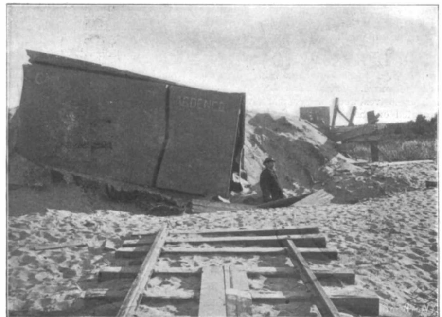
Gathmann Shell Test. Third Round. Target and Backing Driven 8 Feet to Rear and 8 Feet to Left of Original Position. Note Relative Position of Track and Target.
