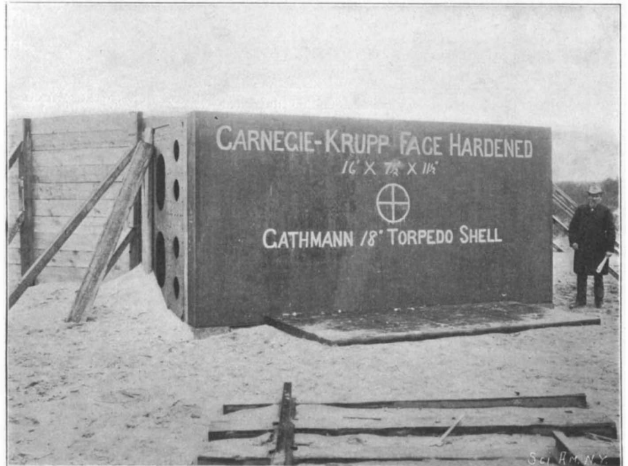
Gathmann Shell Test. Target Before Firing, Backing Representing Side of "Iowa."
