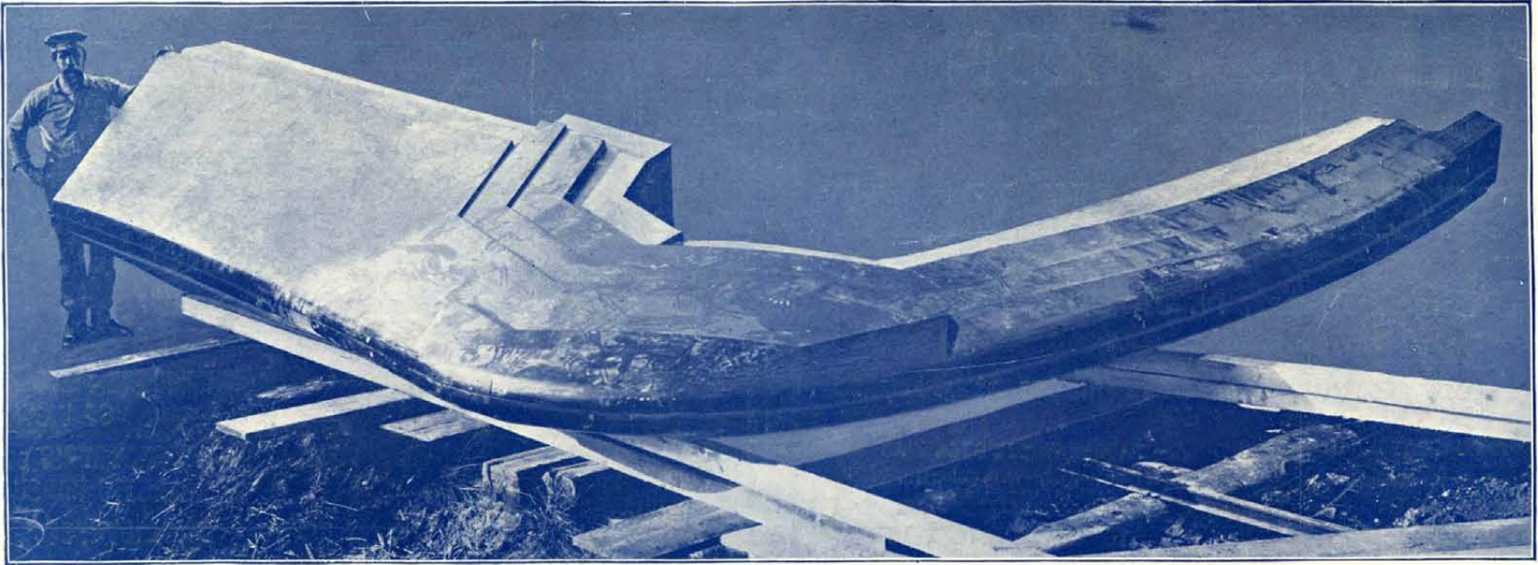
Forty-three-ton Jupiter Steel Castings for the Battleships Rhode Island and New Jersey.
