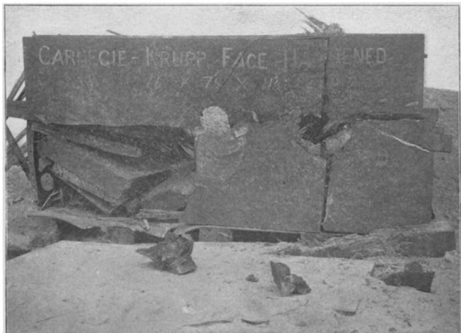
An 11½-inch Kruppized Plate After Attack by Three of Our 12-Inch Armor-Piercing High-Explosive Projectiles. Plate and Backing Completely Wrecked.
