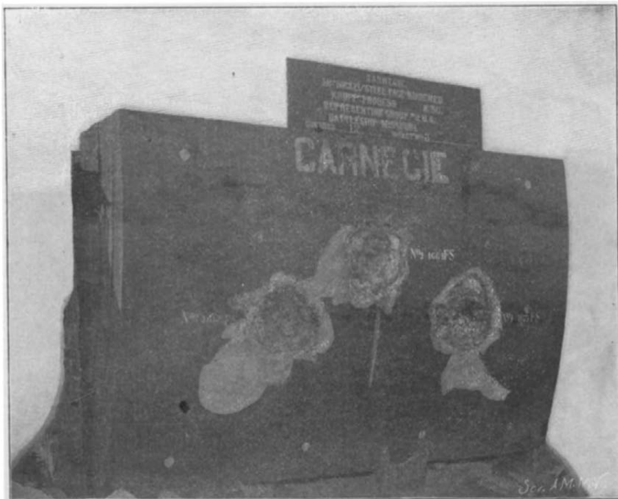
12-Inch Kruppized Armor Plate Representing Armor for the "Missouri," After Attack by Three 12-Inch Shells. Projectiles Smashed on Plate. Penetration, 4¾ Inches, 4¼ Inches, and 3¾ Inches.
