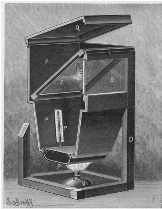
Fig. 2.—DEVELOPING A DAGUERREOTYPE WITH MERCURY FUMES.
