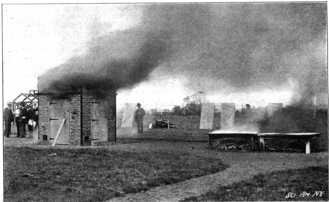
URALITE DOORS OF HUT, RESISTED FOR 1½ HOURS A TEMPERATURE OF 2275 DEG. F., PASSING NO FLAME.
