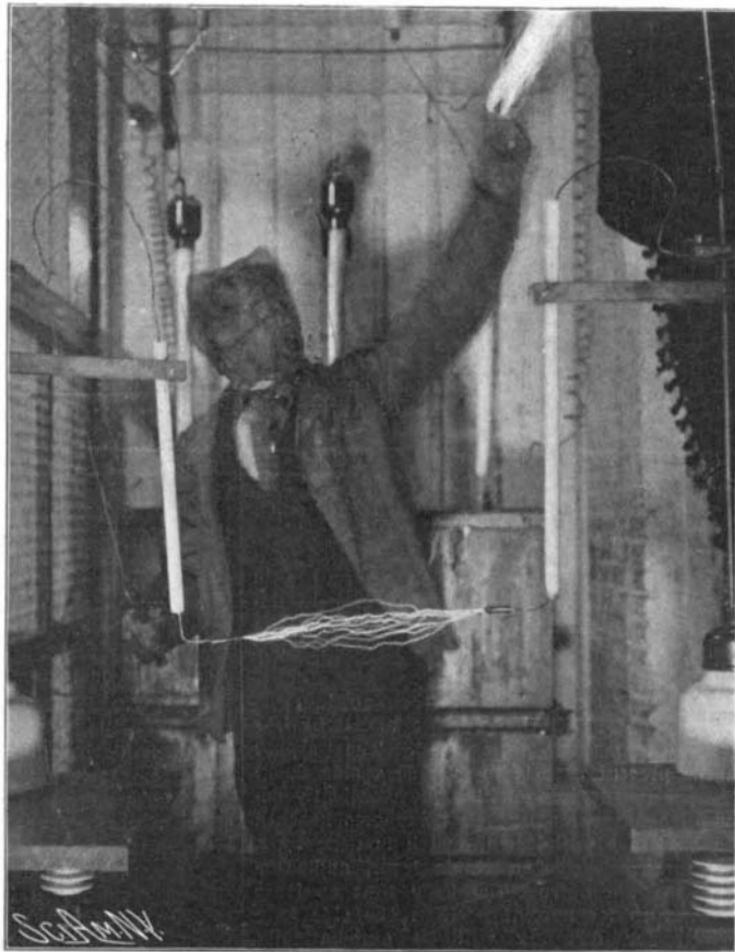
Fig. 1.—THE COAT OF MAIL SHIELDING ITS WEARER FROM A TENSION OF 150,000 VOLTS.
