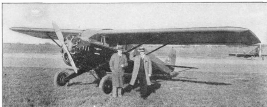
The Aristocrat monoplaner, a three-seater cabin type
