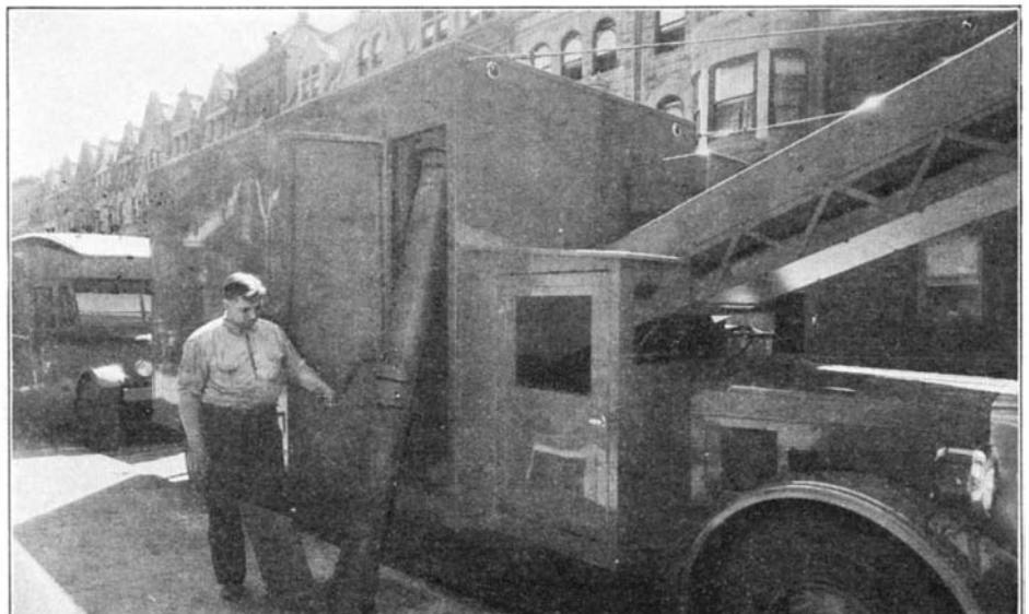
Ashes being carried from a basement to an ash truck by suction. Over the driver's seat is the conveyor which transfers ashes into a dumping truck
