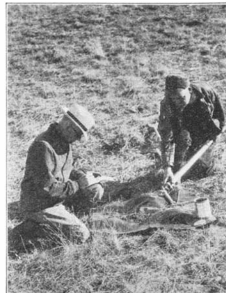
Left and above: Taking samples of soils along a pipeline for use in charting the relative corrosiveness
