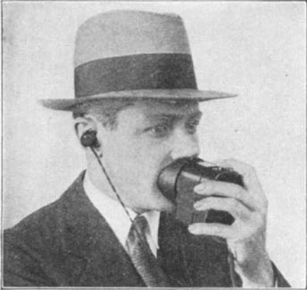
Owing to the high noise level in airplanes, a special type of telephone transmitter must be used. Here is the hand type which has been developed for this use
