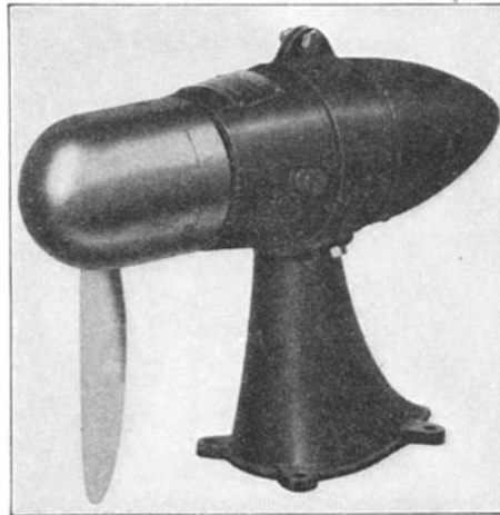
A single-blade wind-driven generator of the type used to supply filament and plate voltages to the receivers used on airplanes. The speed and output are constant
