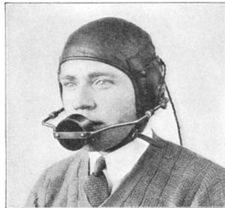
The special telephone set used by the pilots in airmail planes. The receivers are in the helmet
