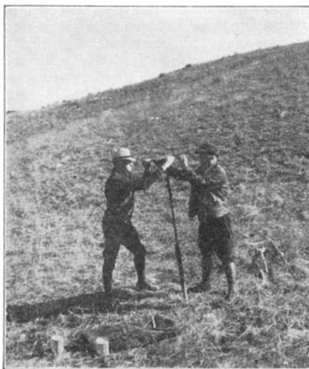
Left and above: Taking samples of soils along a pipeline for use in charting the relative corrosiveness
