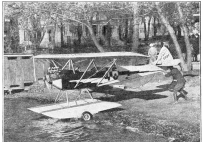
cylinder air-cooled motor. This plane is also available with a wheeled landing gear for land operation
