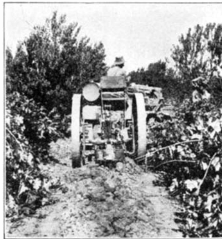
Sub-soiler in operation in a vineyard. The sub-soil is loosened but the surface soil is hardly broken
