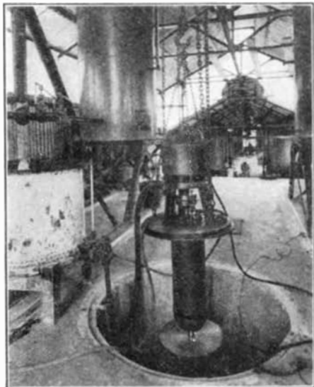
A latex spray-drying unit in a plant on the eastern coast of Sumatra
