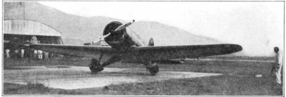
Above: Colonel Lindbergh's new plane with cowled air-cooled engine. Below: The Sirius in flight
