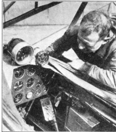
An airplane cockpit equipped for experimental flights under conditions simulating flying in fog
