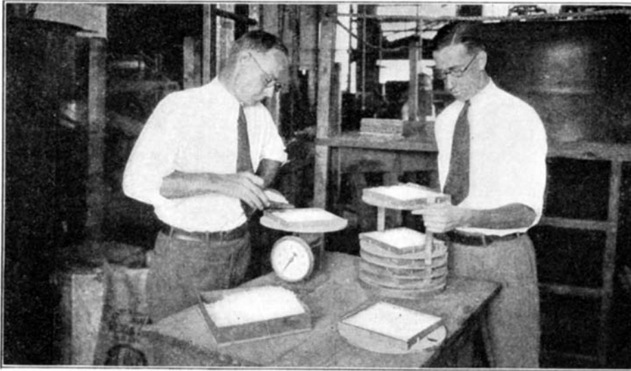
Weighing quartz crystals in the trays in which they will be melted to form window panes, and loading the trays on the holder for the electric furnace
