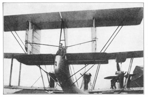
Protecting the vulnerable point. A machine gun in the tail of a bomber
