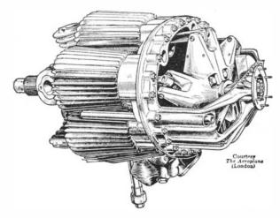
In this view of the Redrup axial engine for aircraft, the fivepointed star member which rotates on the Z crank (the special form of the crankshaft) may be seen at the right end. The cylinders lie parallel to the centerline of crankshaft rotation, as explained in the accompanying text
