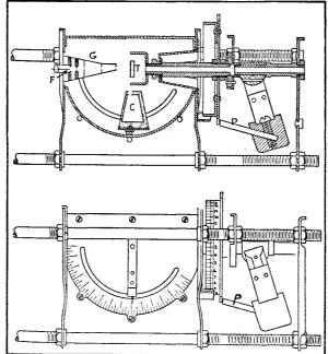
The actual apparatus devised by Davisson and Germer for exploring in three dimensions the space surrounding the target T of electron gun G. Angle of electron collector C, may be varied by means of curved slide; also target can be rotated (see dial on lower section drawing of same apparatus). Galvanometer connected to collector C registers the number of electrons
