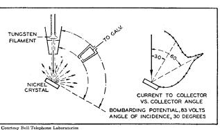
In measuring electron scattering, the "electron gun" at upper left corner sends a steady stream of electrons to the crystal, which scatters them in various directions. The collector (marked "to galvanometer") catches more or fewer electrons according to its position. In the case at right, for example, the maximum number of electrons caught was at 60 degrees angle. This is the principle of the method used by the physicists Davisson and Germer of the Bell Telephone Laboratories
