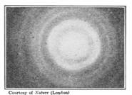
In the author's experiment rings were produced on a photographic plate by electrons scattered systematically in passing through a gold film. The pattern is interpreted as due to electron waves. See the text, page 40
