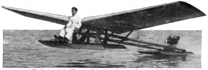
The fuselage of the "Waterplane" rises from the water after a run of 150 feet
