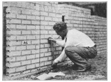
stitute. At right, an assistant makes use of the strain gage, sensitive to 0.002 inch, for measuring shrinkage
