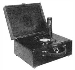
The photoelectric cell is an important part of this light meter
