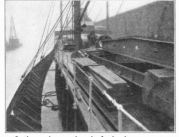
Steel cargo battens close the five hatches; ten steam winches discharge the paper at a rate of 200 tons an hour
