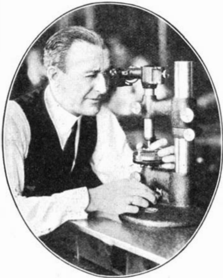
Checking parallelism of film sprocket faces. Microscopic measurements are made of all of the parts
