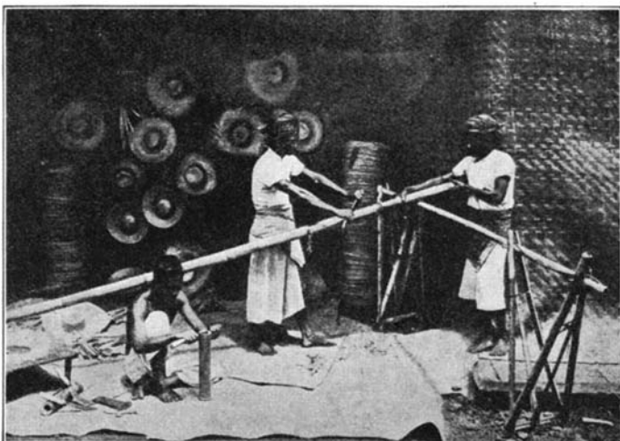
Bamboo is harvested before the branches bud, cut into lengths of six or seven joints each, and then scraped
