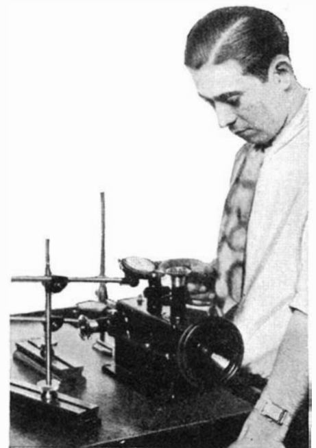
An optical system being adjusted. A highly accurate beam of light is required for film reproduction
