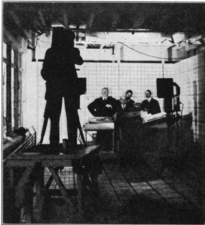
Studying less fatiguing methods of work by means of the moving-picture camera set up in a manufactory
