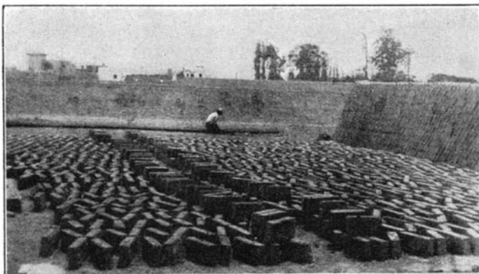
"Not a boundary wall." Piles of bricks ready for use and others drying in the sun at a native brick "factory"
