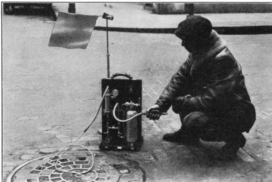
The gas detector which measures the accumulation of deadly gases in sewers
