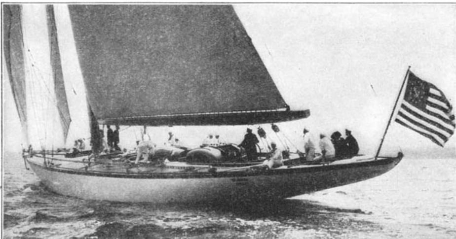
Deck view of the Whirlwind . She is a double ender with canoe stern. This is the first time this form of stern has been used in an America's Cup yacht
