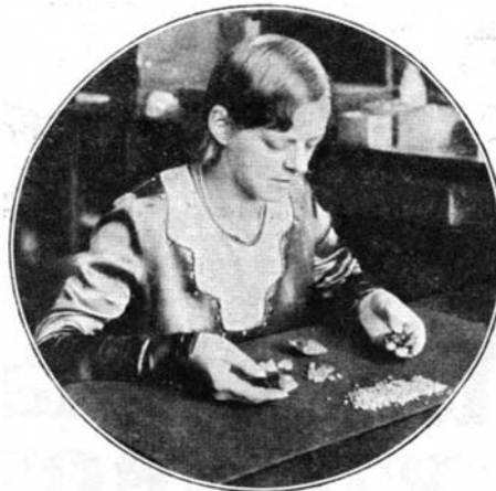
Rough sapphires, synthetic and natural, are sorted by cathode rays
