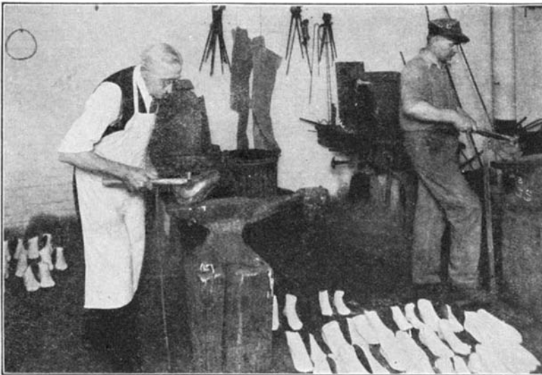
In this picturesque forge shop the iron plates are made to conform to the plaster replica of the foot made in the mold
