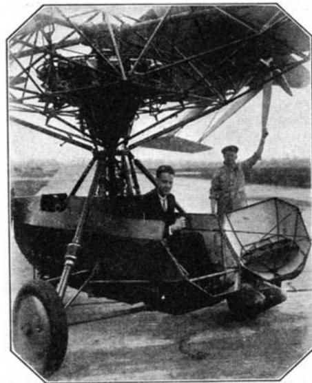
Cock-pit of the helicopter, showing connection of engine and body
