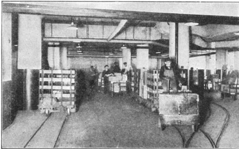
Shipping room of a large commercial house showing how freight is loaded on to tunnel cars
