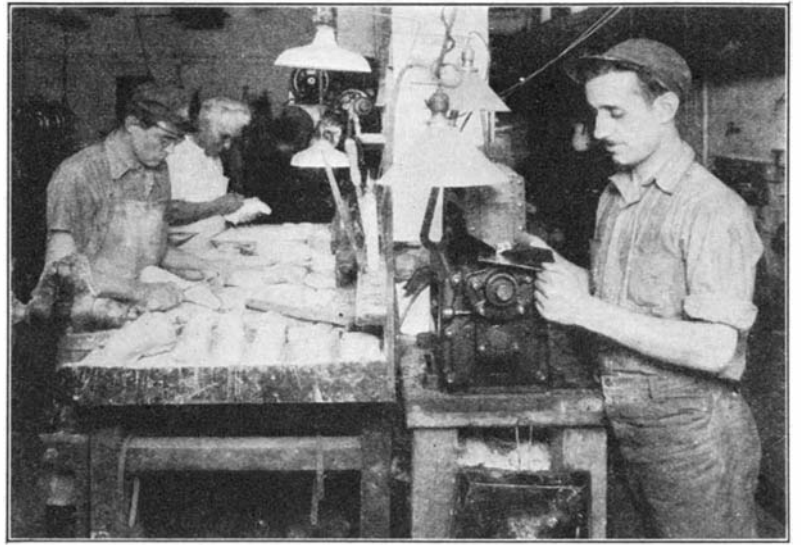
A plaster duplicate of the crippled foot is cast in the mold, trimmed, and a piece of metal is cut to shape for forging
