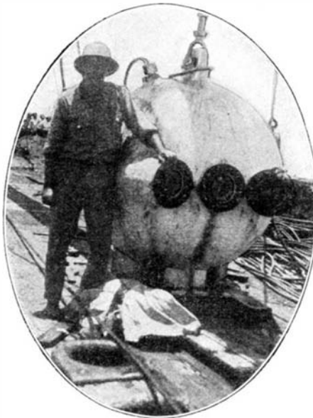
Two of the three windows are closed by heavy three-inch quartz plates
