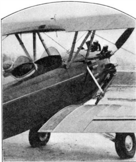
Two complete sets of instruments and controls are mounted in the cockpits of this new sport trainer
