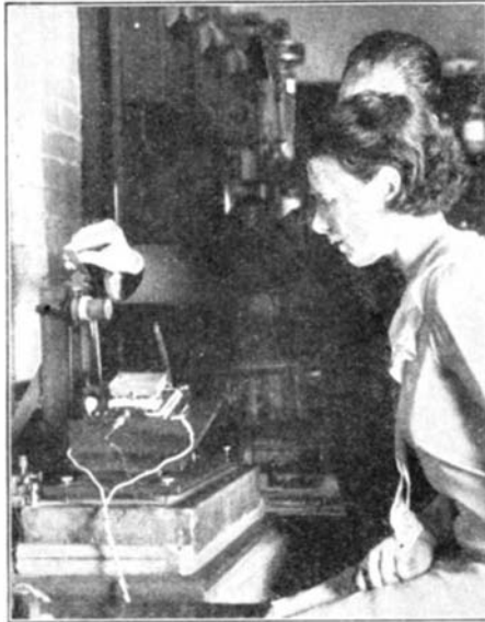
Demonstrating a device designed to measure the oilyness of oil
