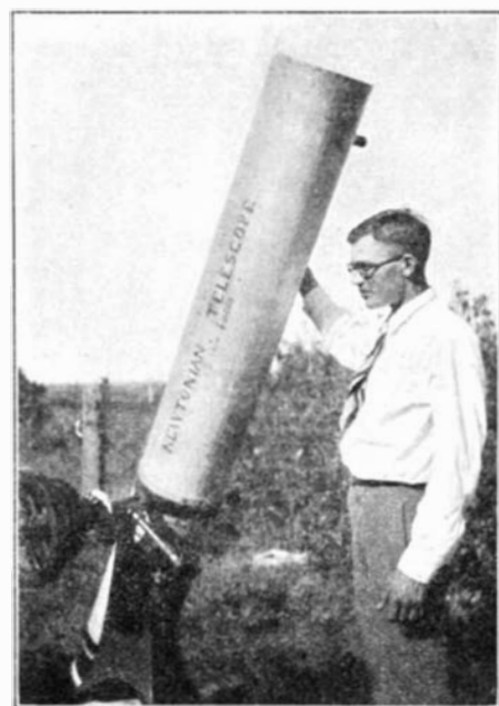
The author standing beside his nine-inch home-made reflecting telescope described in this article
