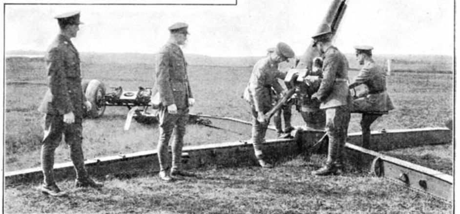
With outriggers spread and wheels removed, the gun's traverse is 360 degrees; its elevation 90 degrees
