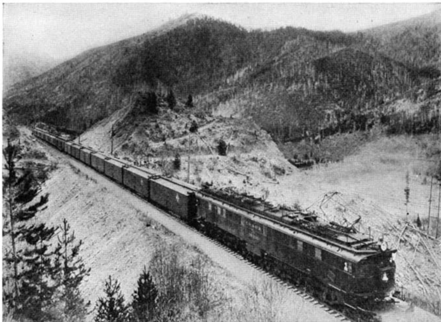
A crack silk train of the Chicago, Milwaukee, and St. Paul drawn by a 300-ton, 3000-volt direct current, Baldwin-Westinghouse electric passenger locomotive
