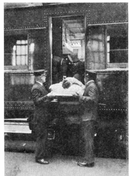
The loading and unloading of invalid passengers bound for the Mayo Hospital is rendered easy by the side doors which permit the direct transfer of the patient on a stretcher to the car
