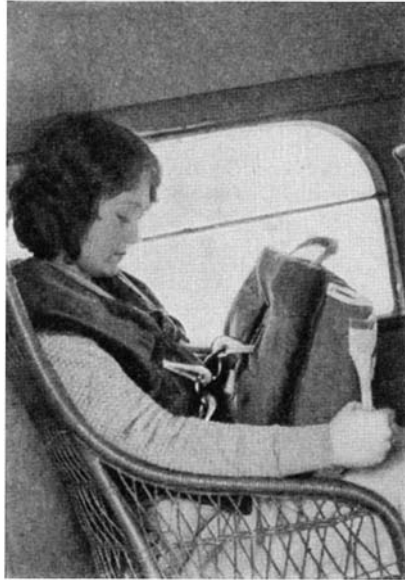
Seated within the cabin of a large airplane, the young lady above wears the parachute harness which is covered with a velour jacket. At right, she has snapped the simple parachute hook into the harness ring
