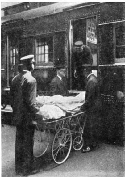
The loading and unloading of invalid passengers bound for the Mayo Hospital is rendered easy by the side doors which permit the direct transfer of the patient on a stretcher to the car
