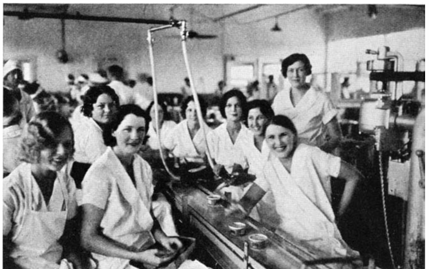
Georgia peaches, to be frozen in the cartons on the conveyor in front of the girl workers, have a sugar syrup added to them from the rubber hose overhead
