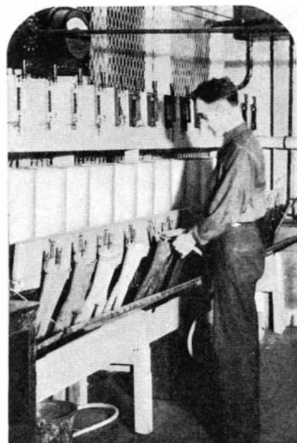
Filling rubber gloves with water as part of an electrical leakage test
