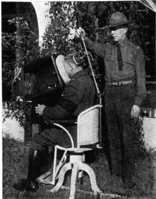
At right: Close-up of instrument box for use with Barany chair to show illusions caused by vertigo. Below: Method of using instrument box with Barany chair. Slide removed in both cases to show instruments
