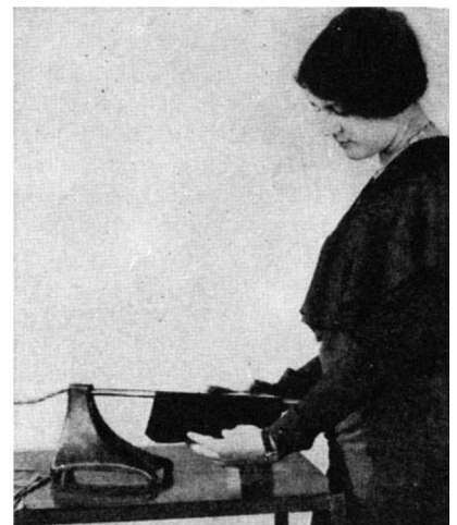
Used carbon paper can be rejuvenated three or four times by passing over an electrically heated cylinder. The saving is worth while
