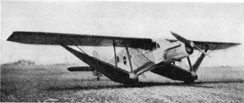
The Bellanca Airbus has a novel system of wing trussing
