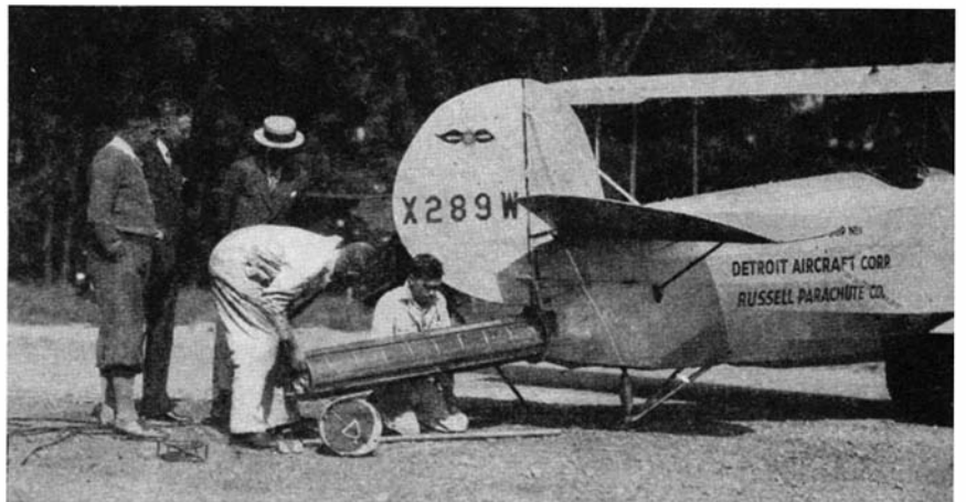
Loading the airplane parachute in the tail of the fuselage. The pilot's chute which is contained in the cup pulls the large 60-foot chute from the cylinder
