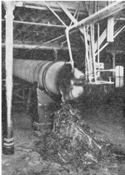
Where tobacco is mixed hot or cold, dry or moist. Capacity 50,000 pounds a day
