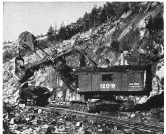
One of two four-yard electric shovels used on the job. Operated by a single man, this shovel loads rocks weighing up to 25 tons on the cars
