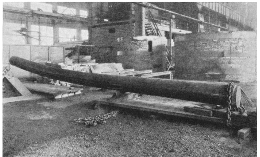
Made airtight, the curled section shown above is subjected to high pressure. It slowly uncurls and finally ruptures at five times normal working pressure
