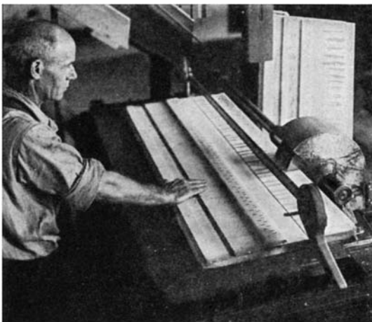
The board with the ivories glued thereon is separated by saws to form the individual keys
