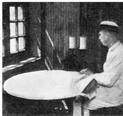
The refinery "seamstress" is sewing cloth on the leaf of a filter press
