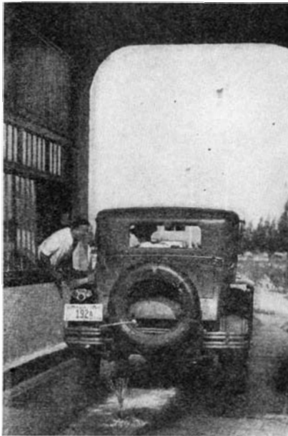
A piece of cable imbedded in concrete "grounds" the static of a car
