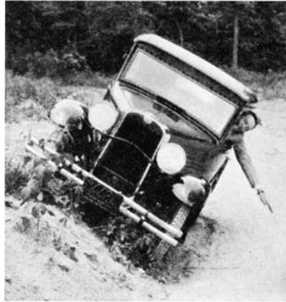
Its low relative center of gravity gives to the Austin great stability
