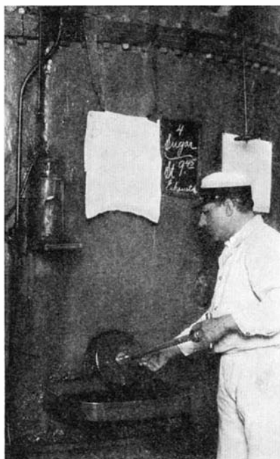
The "sugar boiler" is taking a test sample without loosing the vacuum
