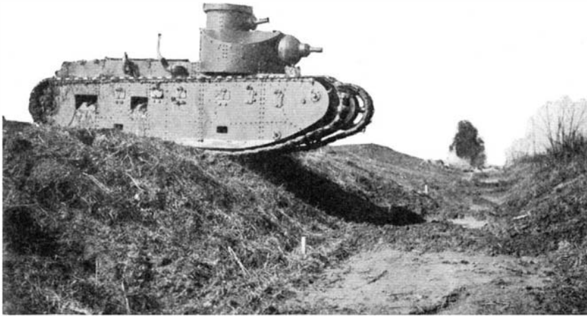
A medium tank entering a trench in a Proving Ground test. A recent development, this tank is formidable, speedy, and not so cumbersome as wartime heavies
