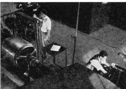
This isn't a dynamo in the left of the picture; it is a dynamometer which measures the pull on the rollers under the wheels of the car.
