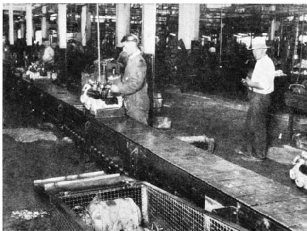
In the factory the tiny engines are assembled on a conveyor table which carries them to the general assembly
