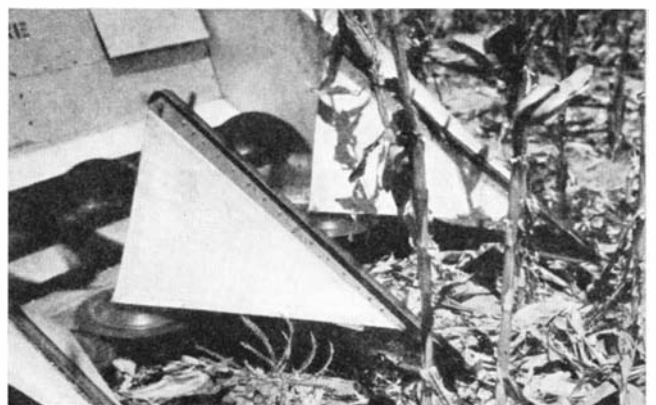
Pointed deflectors turn the corn stalks in toward the rotating disks with sharp serrated edges which cut it easily
