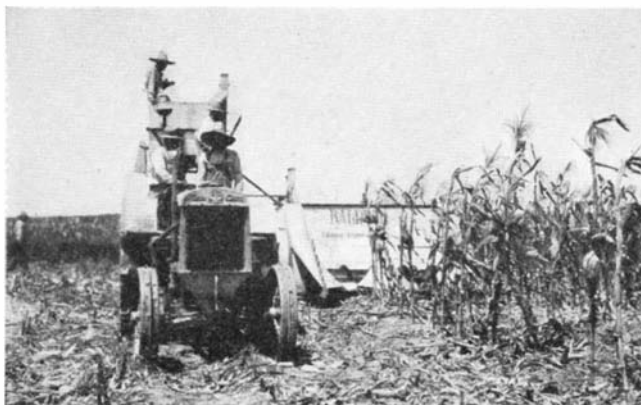
A tractor pulls the corn combine which harvests corn, shucks and shells it, and dumps the shelled corn into bins
