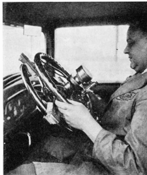
The mechanism which determines the turning radius of a car as it is tested
