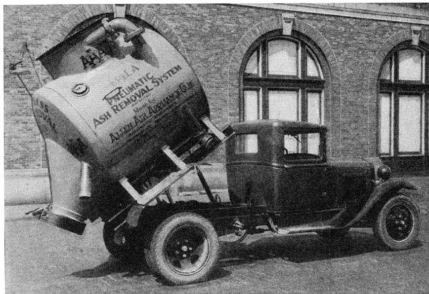
The ash dump unit which, when filled with ashes, is driven away to the dumping ground. Another dump unit takes its place so there is no loss of time
