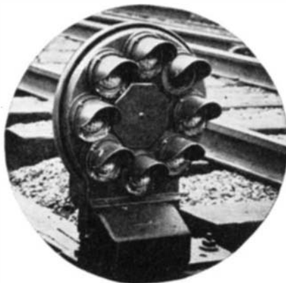
An electric dwarf signal with eight lights can give many instructions
