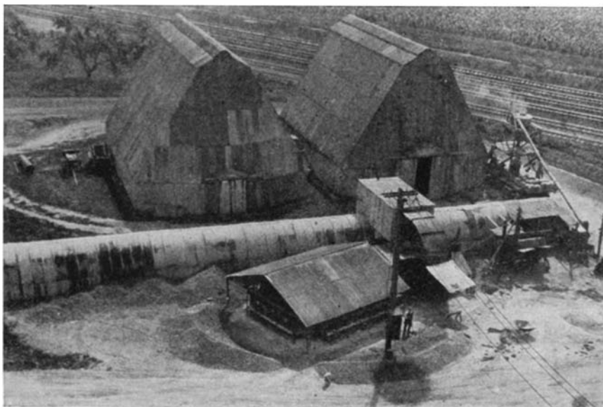
The dehydrator is 40 feet in length and 7 feet in diameter. Green forage enters at one end and emerges dry. At night or when idle it is used for drying manure
