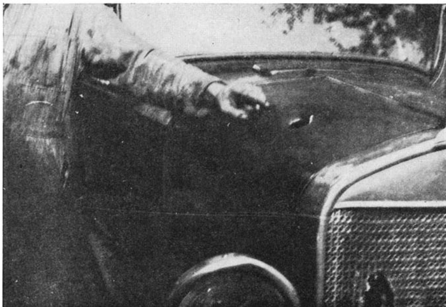
Lawrence Swank pointing to the upper hole. Note other hole in radiator. A meteoric stone of this size would normally not penetrate the hood. Despite the high velocity of meteors when seen aloft in flight, small ones quickly slow down on encountering the atmospheric cushion. When the acceleration of gravity is balanced by air resistance they reach a practically uniform "terminal velocity" which is not high. The probable joke played on Swank rebounded to half of the nation, for it can be demonstrated that millions of persons were given the meteor explanation through the combined circulation of the numerous periodicals which accorded publicity to the original account, despite its unscientific earmarks
