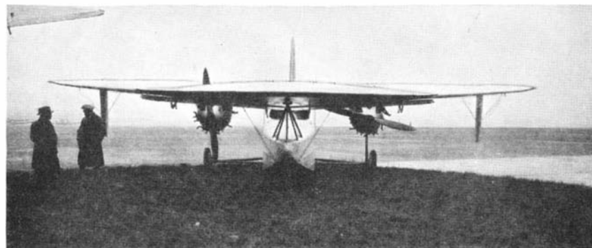
The front view of the Ente shows the abnormally wide landing gear, with struts running directly to the engine nacelles. Note the vertical fins near wing tips
