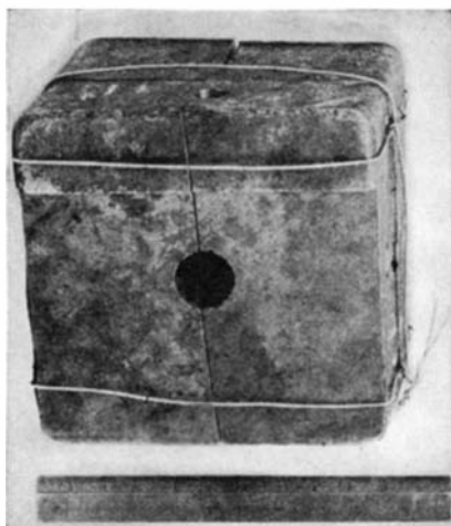
Figure 5: Above; Block of cast iron with large hole leading off one face. Assembled after cutting. Right; Radiograph of casting shown above. Below; Cast-iron block cut to show hidden defects described in the text
