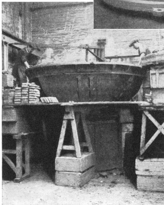
Above: A bell-shaped sand core is built up on a brick center. Left: An iron case or outer mold is lined with damp sand
