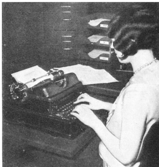
The slightest touch actuates the mechanism; everything is moved by the motor-driven roller
