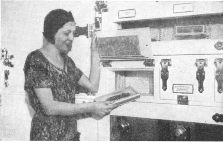
The customer is buying a packaged steak from a refrigerated unit. Another steak will take its place, being lowered by endless chains
