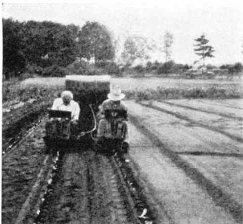
Rear view of the automatic, self steering plant setter showing method of operation
