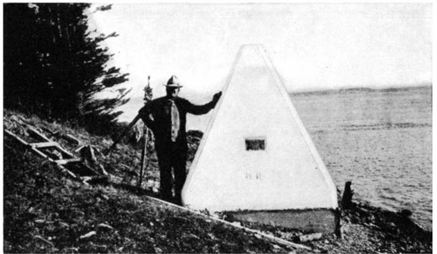
A monument at Passamaquoddy Bay, Maine. To it is referred a point on the United States-Canadian boundary, which is out in the middle of the bay. Triangulation is of decided value in locating various political boundaries
