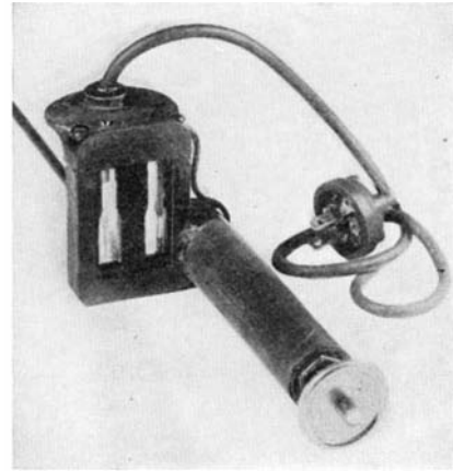
Above: Pump and comparing chamber for determining the amount of sludge in engine oil. Right: The installation being used
