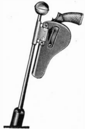
A handy revolver holster that clips to the gear-shift lever of a car
