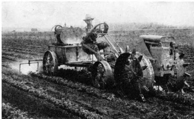
A large size, riding-type powerful garden tractor is used to advantage for pulling an efficient field crop spraying outfit
