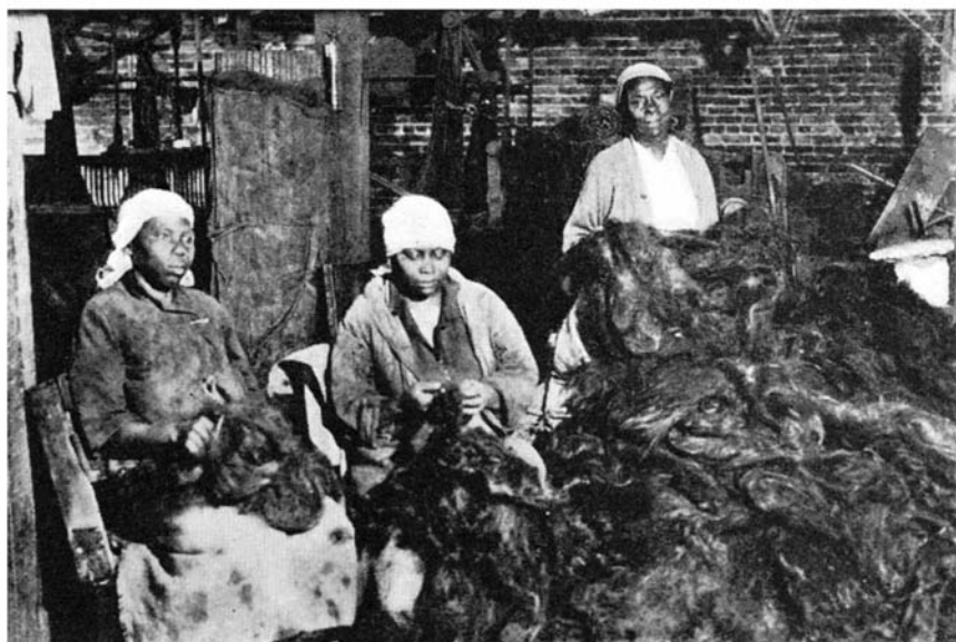
Upper left: A piece of press cloth and a hank of Chinese hair from which this material is woven. Above: Sorting a shipment of hair at a press-cloth factory
