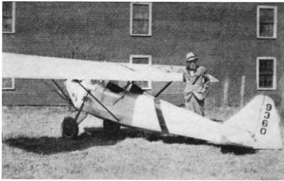
The tiny Heath Parasol plane, one of the smallest in use in America today. It carries only the pilot
