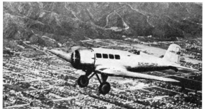
The low-wing Northrop Alpha, with accommodations for six passengers. The pilot's open cockpit is in center
