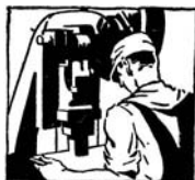
Preswood can be punched or die-cut with ordinary punch press; no special dies or clearances needed
