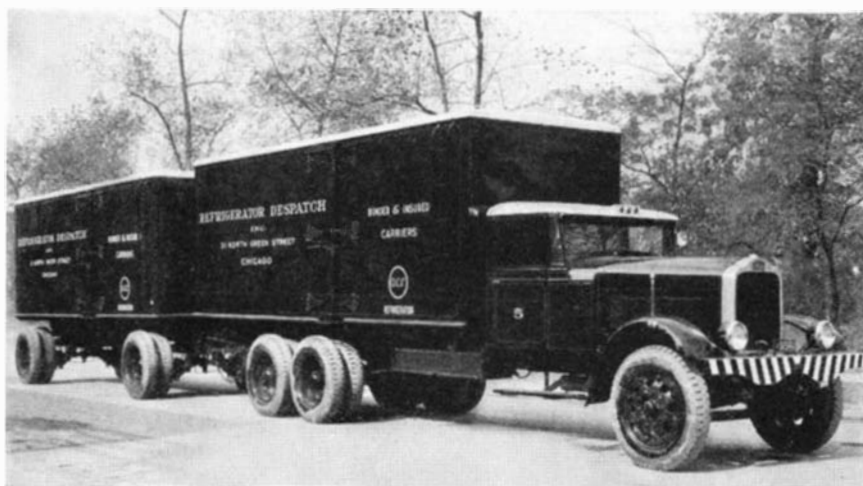
This truck and trailer highway transportation unit has a total capacity of 20 tons. Six hundred pounds of Dry-Ice maintain a constant temperature. If a similar unit were designed for ice, about 6000 pounds of ice would be required
