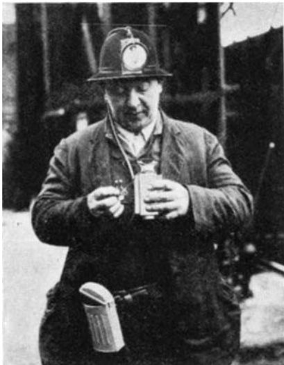
Demonstrating the self-rescuer. Note nose clips and mouth grip
