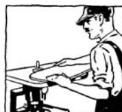
Preswood, with the ordinary shaper, can be quickly given irregular outlines
