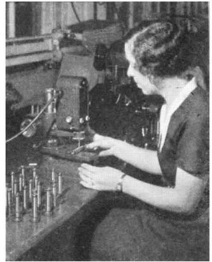
Green, amber, and red lamps on this gage tell the operator the condition of the part inspected
