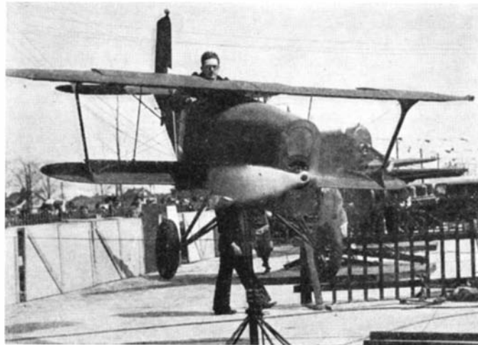
Flying—on the ground! A novel training device that climbs, dives, stalls, and banks, but "keeps one foot on the ground"
