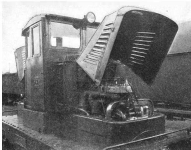
One of the two types of 12-ton locomotives; and below: Standard Mack engine beneath the hood
