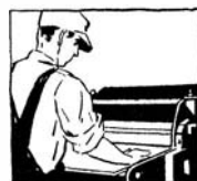
Preswood, when planing is required, needs no special machinery
