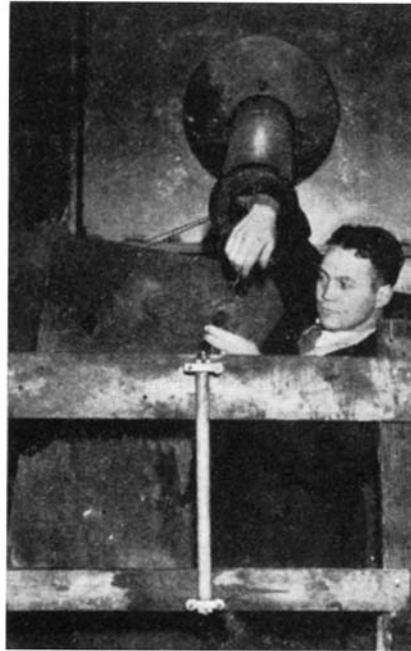
Above: Preparing to test a new lightning rod with "man-made" lightning. Right: The bolt has landed but the Torok lightning rod has delivered a knockout blow
