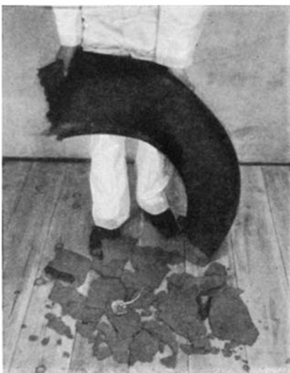
Vulcanized to an ordinary tube, the new truck tire tube resists heat while the other tube deteriorates
