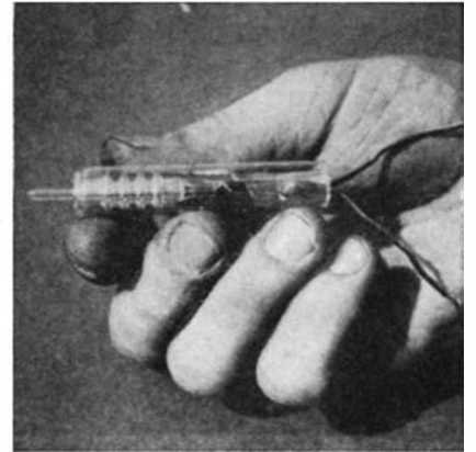
The delicate little tube which controls powerful electrical circuits
