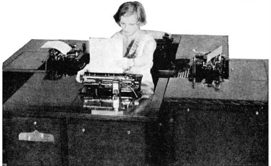
One girl does the work of 12 typists in writing personalized letters. This typist operates four pneumatic typewriters with perforated rolls
