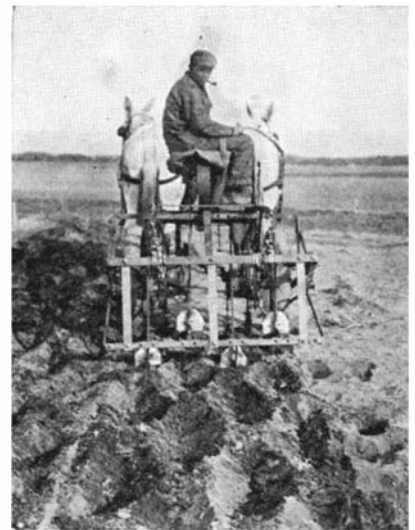
Designed by the U. S. Department of Agriculture to prevent soil erosion, this machine uses sets of shovels which alternately operate to dig holes at regular intervals. The machine digs about 10,000 holes per acre. Rain water stays in these holes, two or three gallons in each, and soaks into the ground instead of running off
