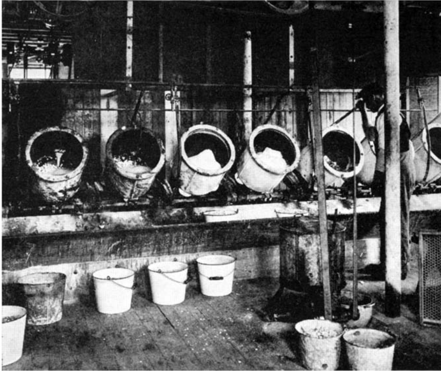
Part of the equipment necessary for the button polishing operations. Finished buttons are agitated in various solutions to bring out their luster.
