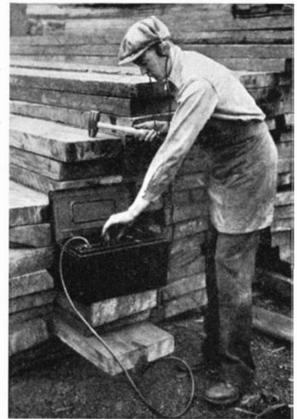
The knife edges on this "electric hammer" sink into the wood and make possible the test described
