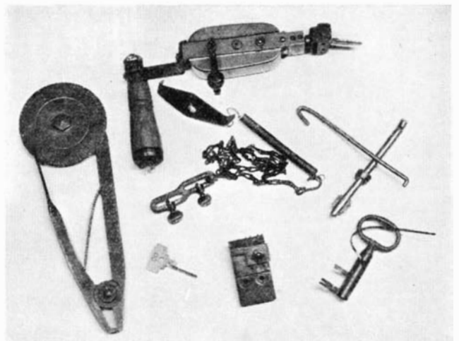
At left is a depth gage. At top will be seen a "tumbler rattler" for raising pins in a pin-tumbler lock. The "gear" belongs to it. Upper right hand device is an extemporized key to open a "bull" pen. Key is pick lock, metal ribbon being fed through barrel to locate the tumblers
