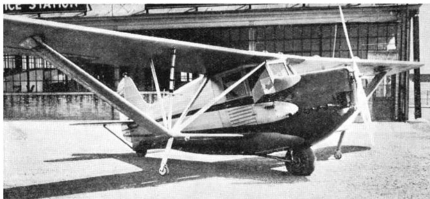
A novel single-wheel plane designed by Charles Ward Hall
