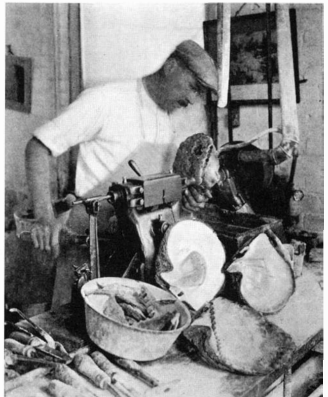
The machine age method of cutting pearl button blanks. Much skill is required to cut these properly so that there will be the least possible waste. Below is shown a large shell with the button blanks cut partly through
