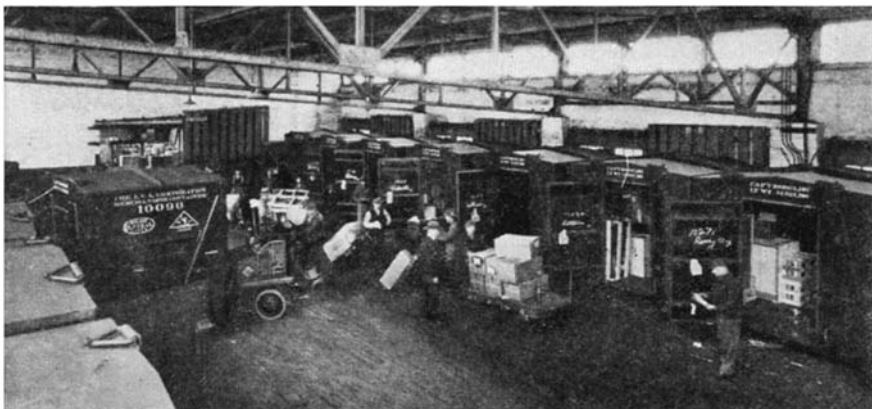
Here is shown a busy freight exchange station at an important junction. The movable containers present an easy way of classifying freight for all stations
