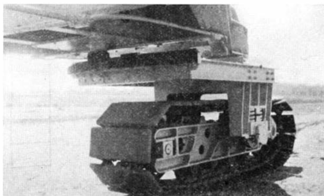
The crawler with which the mast is steered is secured to a saddle casting on a swivel bearing with heavy king pin
