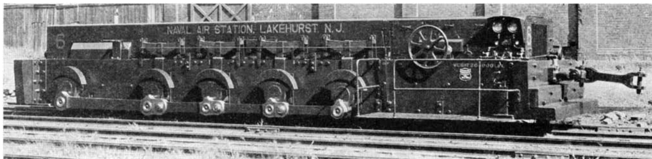
A low, smooth-top locomotive to steer the Akron around its mooring mast
