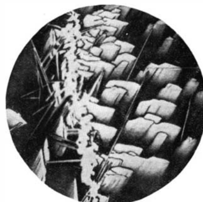
Why is manganese steel brittle when reheated after tempering? At left: What is revealed through an ordinary microscope. At right: Two views at 3500 diameters, showing how reheating caused brittle carbide plates to work into the cleavages and thus destroy the toughness of the steel
