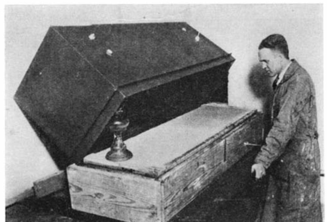
Reducing the intensity of "lath marks" by installing Balsam-Wool insulation in the inner wall space. The wall section at left was insulated; that at right uninsulated
