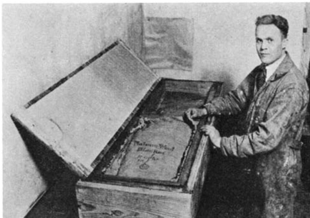
How insulation helps preserve cleanliness of wall surfaces. On the wall section at left, insulated by one-inch layer of Balsam-Wool, the dirt accumulations are almost negligible
