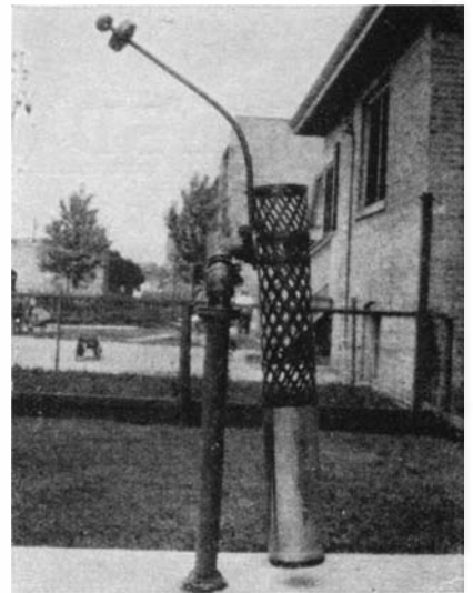
Paul A. Chamberlain's half-and-half reflector with 8-inch mirror
