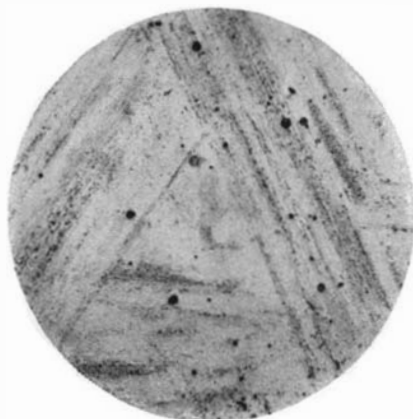
Steel magnified 3500 diameters. The black dots are the ones mentioned in the text—250 atoms wide
