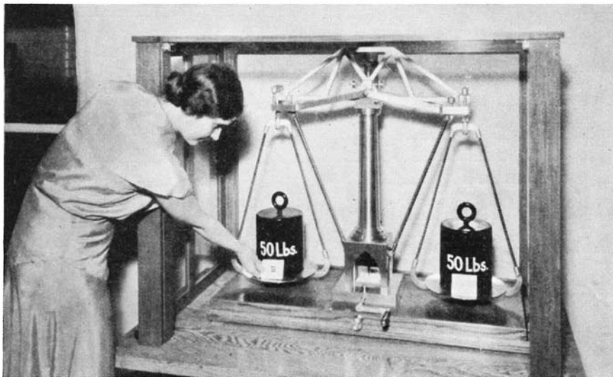
Three pencil marks throw this scale off balance. After balancing weights and pieces of paper, three pencil marks on one paper show the scale's sensitivity
