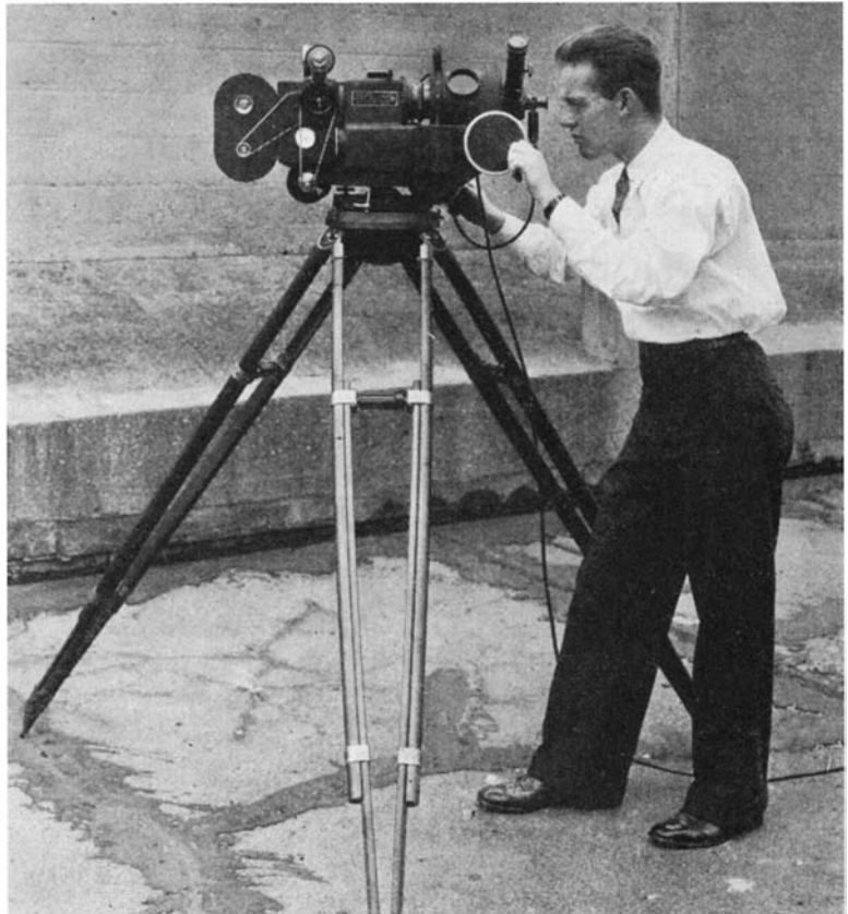
The recording theodolite in action. The operator is training it on the target by looking through the eye-piece and manipulating handwheels. The cable goes to the time interval device and the other theodolite
