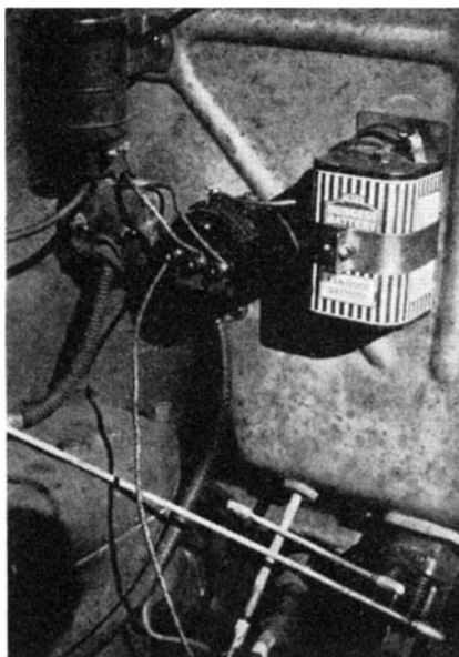
A six-volt dry battery in the ignition circuit assists in starting
