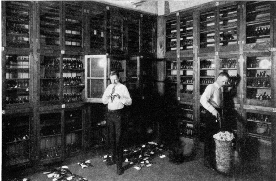
The gun room is a veritable museum of firearms. Examining a revolver and firing a test shot into a basket of cotton waste to preserve markings. The firing range is adjacent
