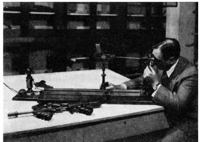
Col. Goddard is examining a weapon from breech to muzzle to see whether it has been fired since last cleaned
