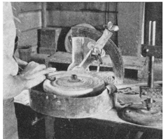
Final polishing is done on a felt lap, holding the spindle in the hands without the meter
