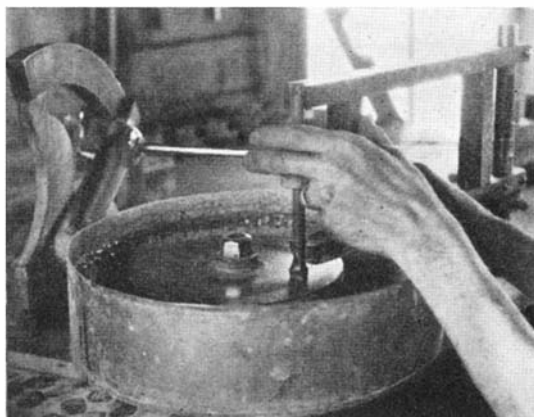
The first grinding is to square the top face and is done with Carborundum on a lead lap
