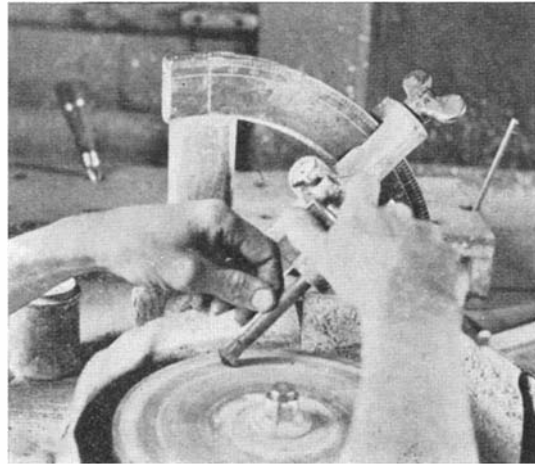
Polishing the facets, aided by a goniometer. Most faceted work is beyond amateur capacity
