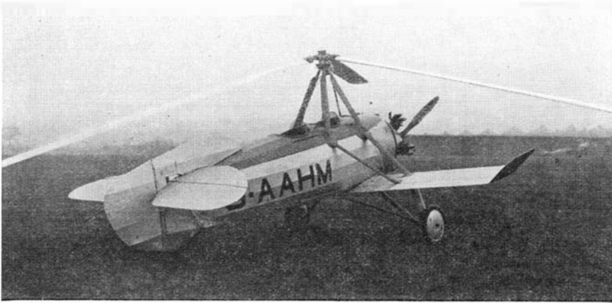
Autogiro in which droop and interblade cables have been eliminated
