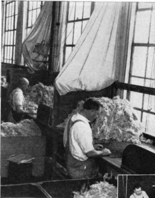
The quality of mohair velvet depends on the care with which fleece is sorted. Skilled sorters can pick out 15 different sorts from a single batch of fleece. It takes three years to become a sorter. A good craftsman can handle 1500 pounds a week with the aid of fingers alone
