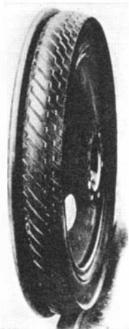
A close-up of one of the wheels of the rail car, showing the flange, pneumatic rubber tire, and rail
