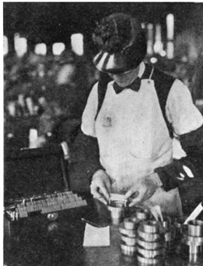
Toolmakers use gage blocks as a quick and accurate means of checking up all kinds of work. Note case of various sized blocks at left
