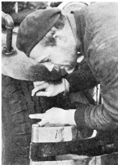
After the 14-day run on the Indianapolis Speedway, the tires of the truck which made the non-stop vehicle record showed little wear
