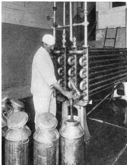
Milk as received from the dairyman is too warm to ship to the city; germs would multiply in it. Hence it is cooled in coils beforehand
