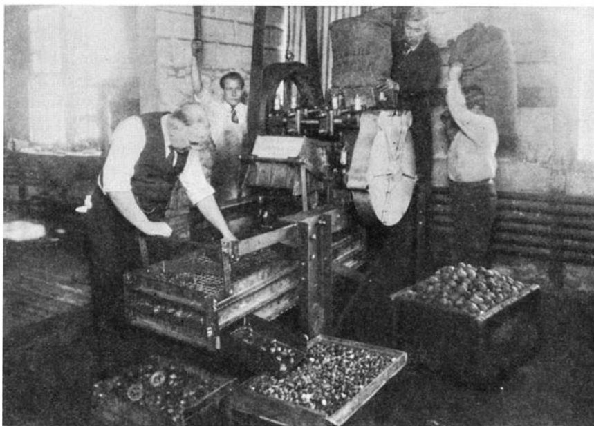
The machine that opens cohune nuts without harming the kernels
