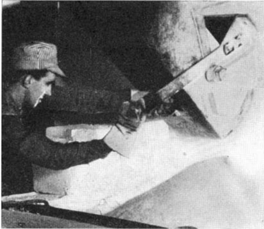
The materials are weighed out and mixed and are shot into the furnace from this chute
