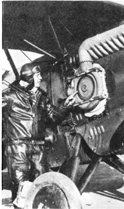
Captain Reuben C. Moffat, of Wright Field, pointing to the supercharger of his Curtiss Conqueror with which he flew, at an altitude of 25,000 feet, at a speed of 266 miles an hour. At right: A diagram of the General Electric supercharger
