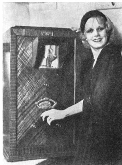
The Freed television receiver and reproducer, showing the shadow box which can be folded downward
