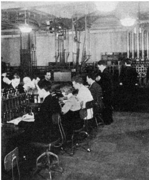
Special wires lead from the room at the right to 40 important offices throughout the country where cable traffic is collected. These wires connect to printing telegraph machines from which the messages go on their way to various foreign lands
