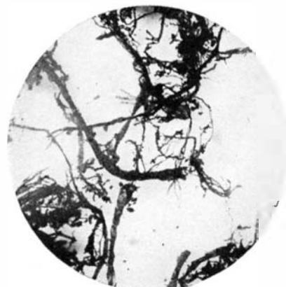
Shredded leather fibers completely disentangled. Note fine tendrils branching off from the main fiber stems. (Magnification is 50 times)
