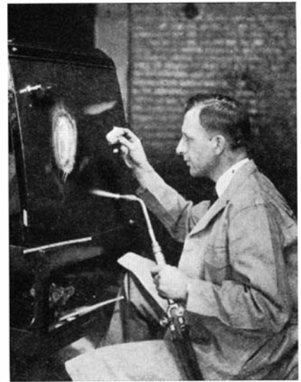
Deep dent in automobile door being filled with new hot-plastic alloy
