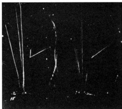
Figure 7: A remarkable photograph of the natural disintegration of atoms, described in the text. The vertical part of what looks like a check mark is a helium atom just shot out of an atom of thorium emanation. Fragment left is an atom of lead and this has a very short track—a tiny stub at the point. Right-hand side of check is track of helium atom. Other check is same event taken at right angles
