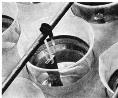
Below: A laboratory set-up to test the corrosion of welded joints, in which the corrosive action is speeded up. Left: Close-up of one of the glass immersion units
