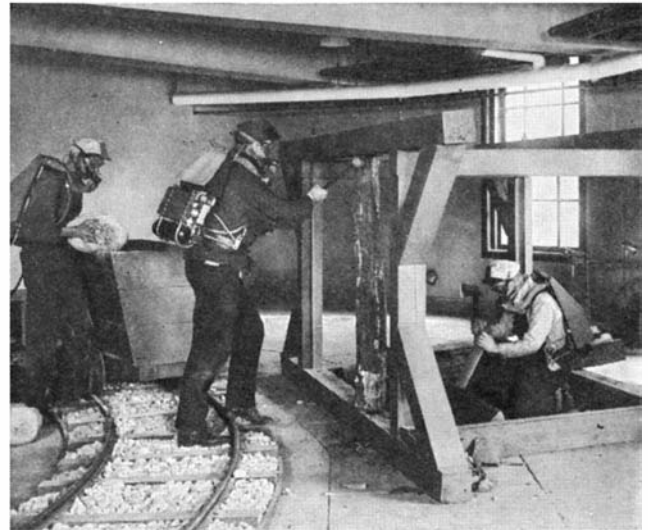
Below: Men being trained at the Pittsburgh Experimental Station with the Gibbs mine-rescue breathing apparatus in an irrespirable atmosphere. The men perform mining operations
