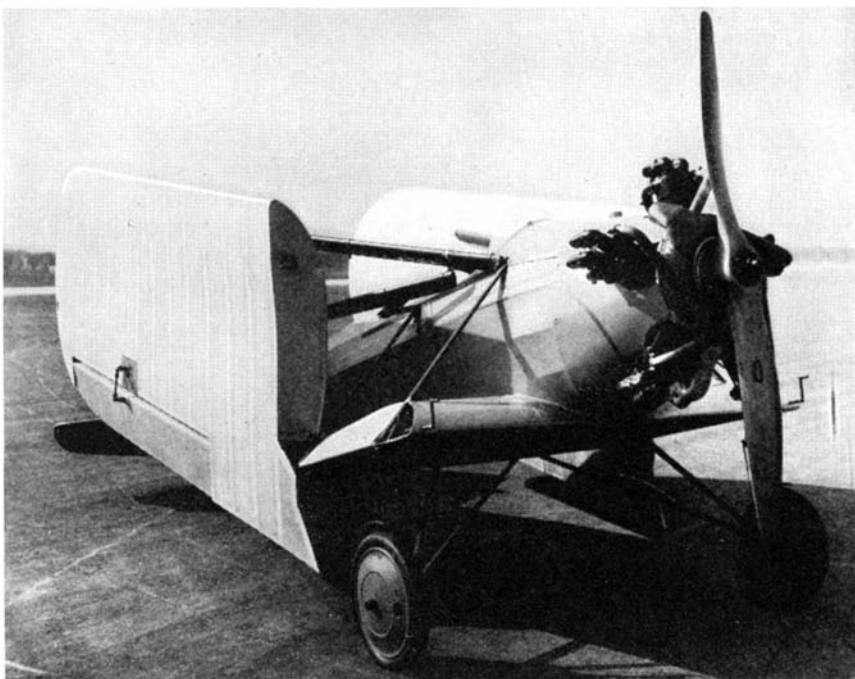
With wings folded, this plane can be stored in a nine-foot space
