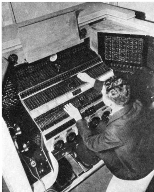
Thermionic light organ for obtaining unusual lighting effects in a hall in Cleveland, Ohio
