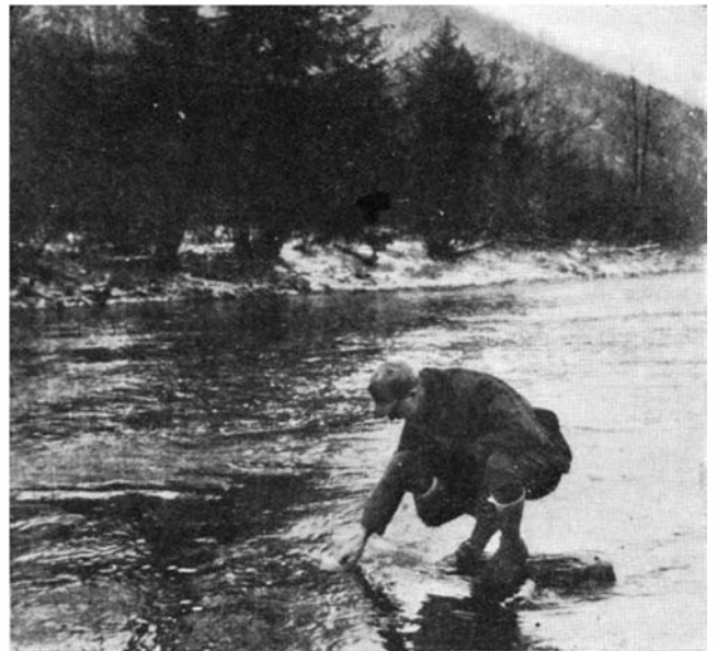
Surveys are made to determine the character and amount of acid water given off by mines so as to note the effect on streams. The man is taking a sample of polluted water
