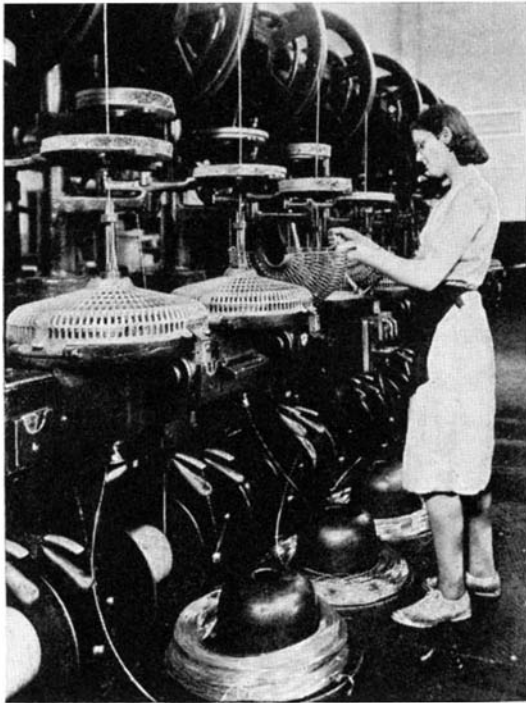
Paper insulating machine applies narrow strips of paper to the copper wire in spiral form
