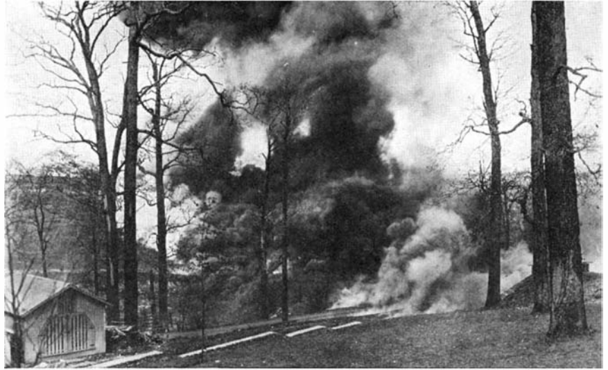
At Bruceton near Pittsburgh is located the experimental coal mine of the Bureau of Mines. Here is shown a violent coal-dust explosion. The white patches in the smoke are flame
