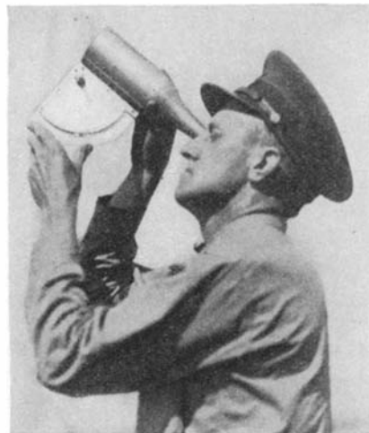
Using the clinometer which indicates the height of the "ceiling"
