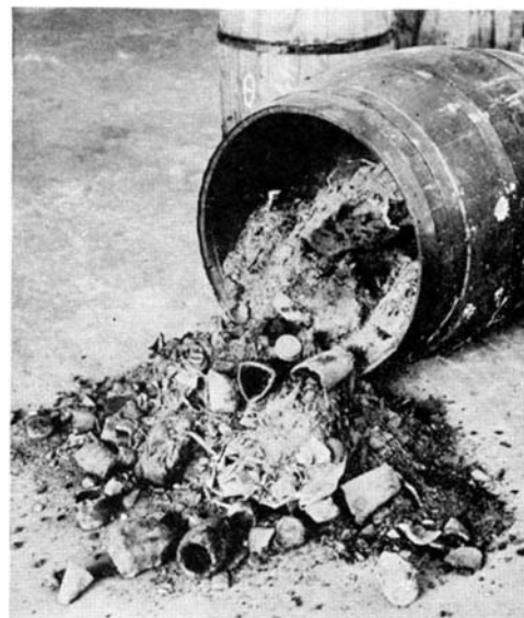
A 5000-dollar barrel of "sweeps" as it is received by the refiner, before crushing
