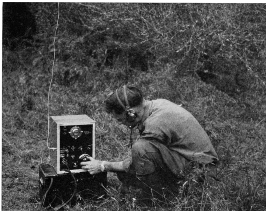
One of the semi-portable radiophone transmitter-receivers set up in the field under actual operating conditions. The aerial is strung between near-by trees
