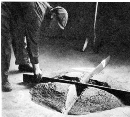
After reduction to powder the mass is divided into four parts for assay by interested parties
