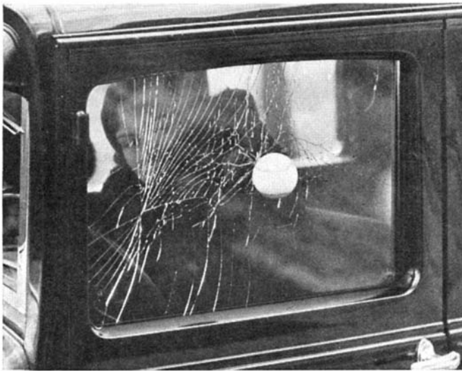
When the safety glass in the door of a car is struck, it will crack badly but will be held together by its sealed-in celluloid center
