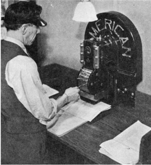
Operator is perforating interline waybills to show station audit number and date of report.
