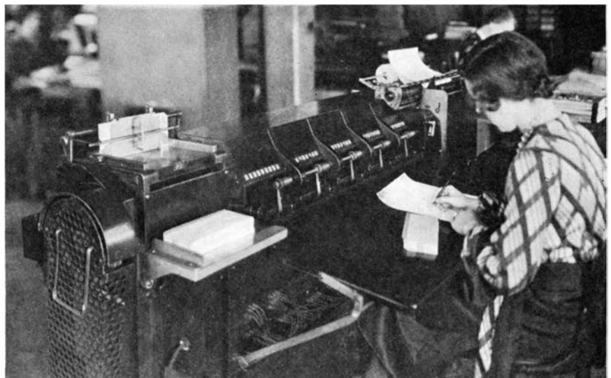
Checking the items totaled by the tabulating machine against the card that has been punched for record purposes, saving much valuable time in auditing
