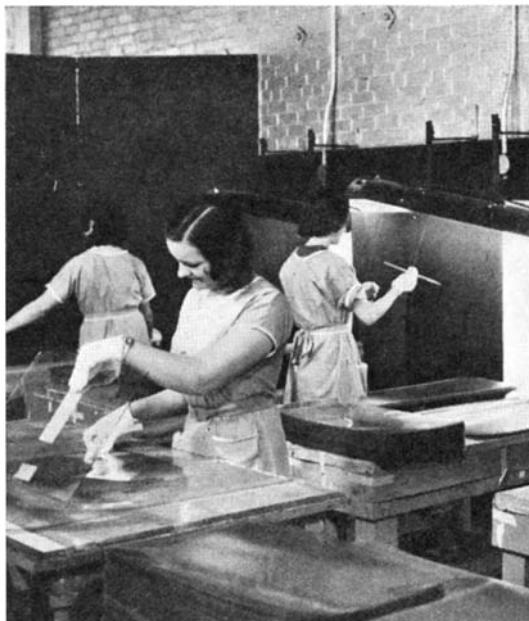
Inspecting pyroxylin for defects, and cutting sheets of it to the outline of a glass pattern
