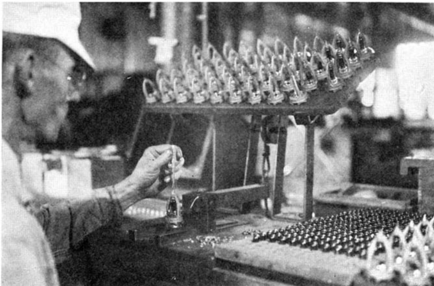
The process of setting quartz bulbs into their frames is very exacting. Note stock of bulbs at operator's right, and frames on rack with and without bulbs
