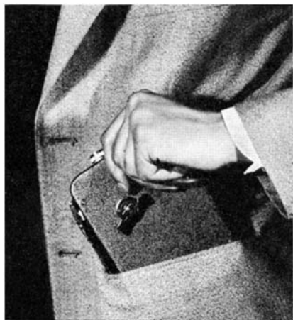
A new movie camera takes four pictures in the space of a 16-millimeter frame, and fits the pocket
