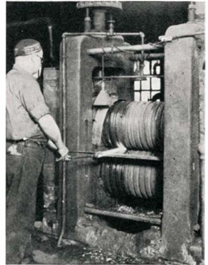
Rolling the white-hot steel to a tapered form for the rifle barrel
