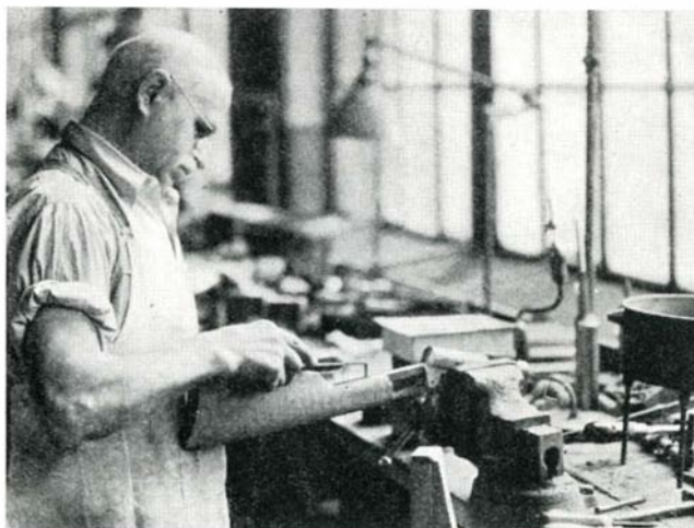
The wooden gun-stock and the receiver are first assembled and then carefully hand-fitted to produce a perfect match
