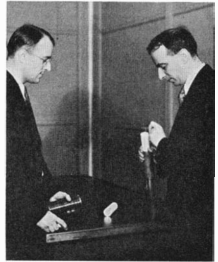
Dr. Slepian showing his new fuse with boric acid as the de-ionizing element. It has just interrupted 20,000 amperes at 13,200 volts
