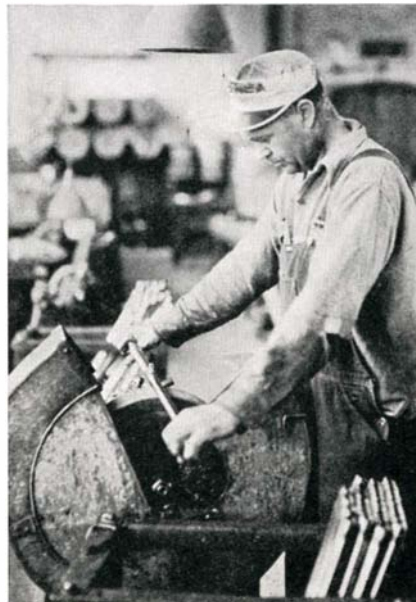
Polishing the outside of barrel on a wheel is known as "spinning"
