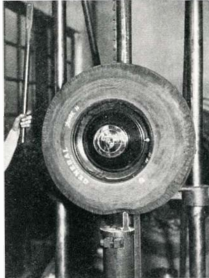
At the left is shown a Jumbo tire in the "pile-driver" ready for the bruise-break test. Dropped repeatedly onto the anvil as shown above, and other anvils of various shapes, the tire sustains many kinds of fabric breaks and tread bruises
