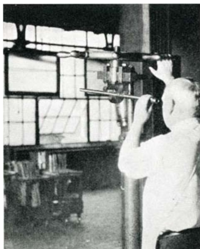
An expert straightening the gun barrel with the aid of a screw press
