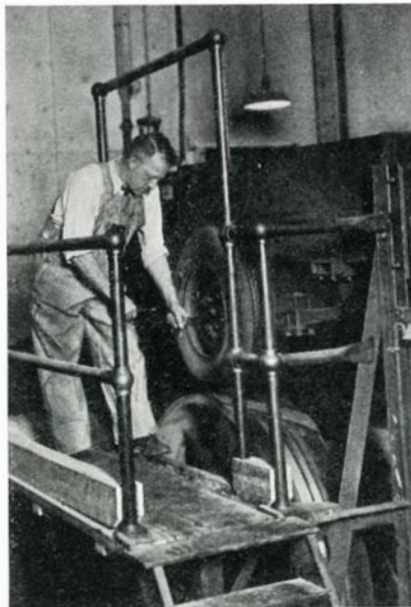
At the right is shown the weight box, used in the pulley wheel test, loaded with several tons of pig iron. Below may be seen the pulley wheel on which a tire is to spin for days, with a cleat over which the tire must bump as the wheel revolves
