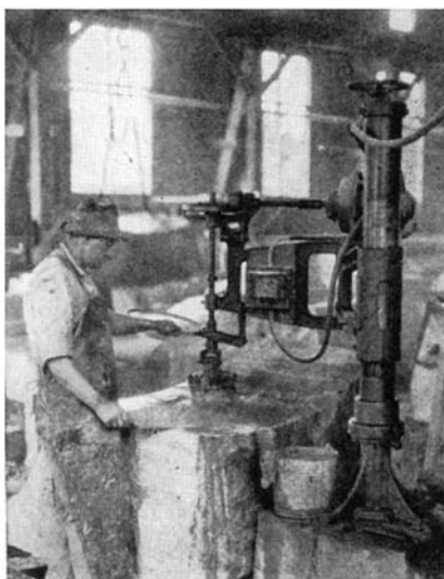
Below: The first polish. A swiftly rotating wheel, mounted on a universal joint and on an arm that may be swung about the supporting pedestal of the machine, will polish the surfaces of almost any kind of curve
