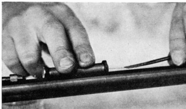
Below: The jewels are threaded on a wire and are held together by the cylinder. Diamond dust is applied; the jewels are polished by rubbing
