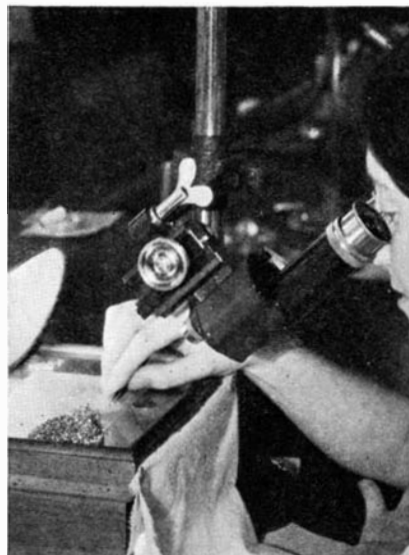
Right: The jewels are individually inspected with a binocular microscope both before and after they are placed in their gold settings
