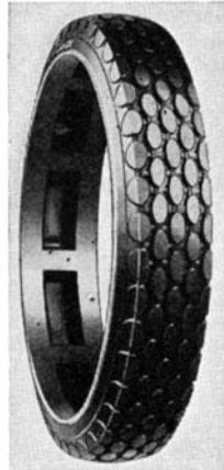
Left: Cross-section of a zero-pressure tire. Above: Tire on steel base
