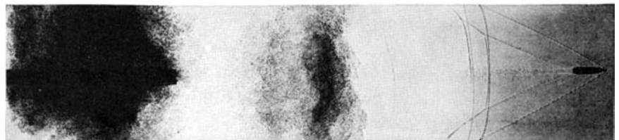
Main volume of gas still acting to reduce recoil as the bullet speeds on
