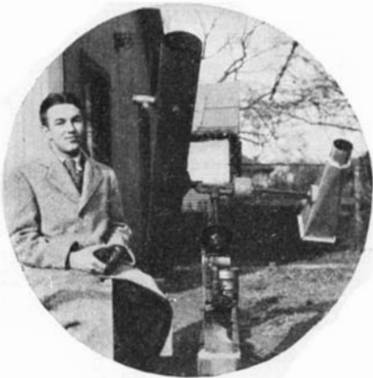
V. E. Maier, 1306 Parker Avenue, Indianapolis, used a camera for a counterweight. His telescope has a phonograph motor drive
