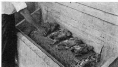
Fowls being placed on the conveyor in the "Z" quick-freezing system
