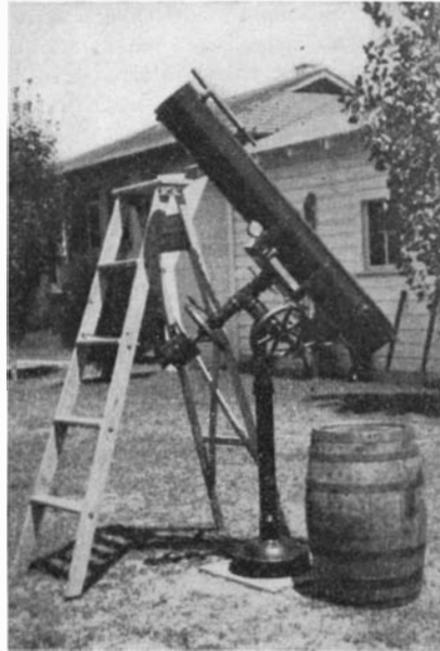
What its maker, Dr. R. A. Pittman, dentist, El Dorado, Arkansas, calls "the thing" is a six-inch reflecting telescope concocted largely from an old Chevrolet brake drum (the base), pipe fittings, and other gadgets. "This mounting has worked very satisfactorily so far," Dr. Pittman states, "and, best of all, the whole thing cost me less than six dollars. The 'observatory' consists of a step ladder and the keg on which the mirror was ground. I sat in one place all during the operation and turned the keg with my feet." Evidently the dentists in El Dorado are mechanics right down to the tips of their toes
