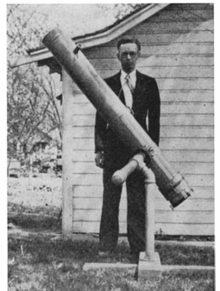
Looking down the skeleton tube of a telescope made, except the 12-inch mirror, by Samuel S. Waters of Indianapolis. The paraboloidal mirror was made by Dr. Loren S. Noblitt
