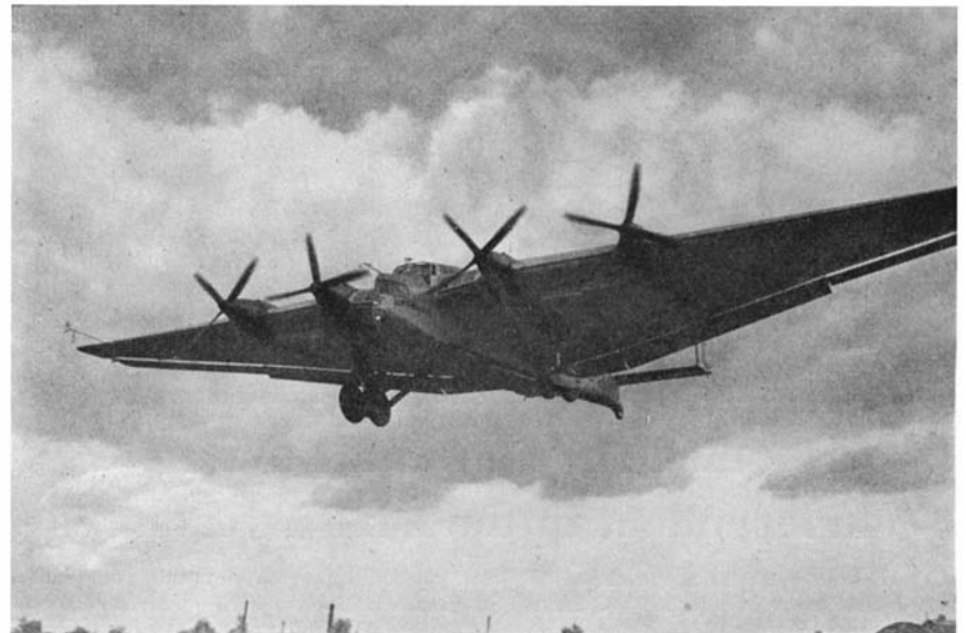
The D-2500 Junkers airliner in flight. The end flaps are ailerons. Note, however, the trailing-edge flaps for slow landing; also compactness of the body
