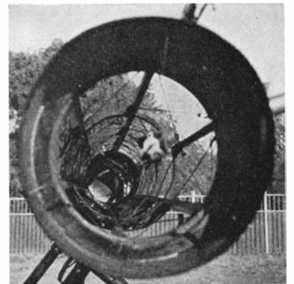
Looking down the skeleton tube of a telescope made, except the 12-inch mirror, by Samuel S. Waters of Indianapolis. The paraboloidal mirror was made by Dr. Loren S. Noblitt
