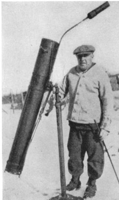
O. E. Stroehlin, Pomeroy Avenue, Meriden, Connecticut, made the concave mirror of his six-inch telescope in spare time during eight days. "This is the first time I have ever tried to make a telescope," he writes, "and it surely was an interesting experience." The post of his mounting is the housing of a Ford drive shaft, and most of the rest is of Ford parts. "The whole telescope, not counting the eyepiece, cost me 18 dollars," he states
