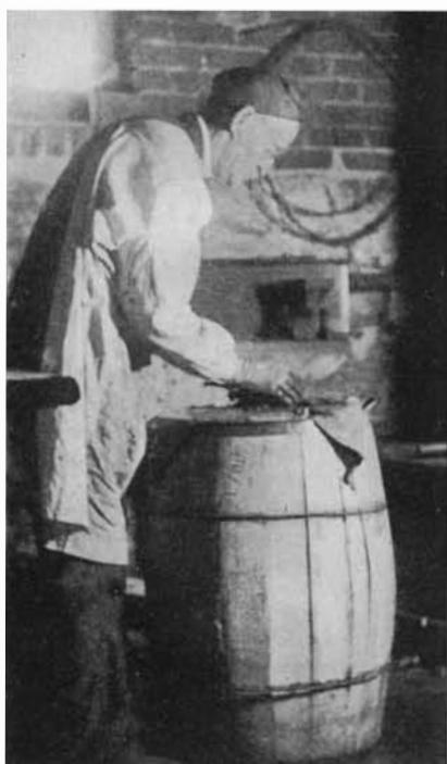
Seventy-six years young and still at it. Dr. George F. Allen of Aurora, Illinois, grinding a mirror
