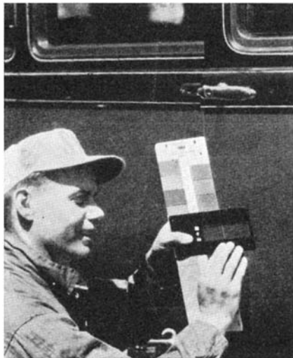
The painter's job is made easy by this new color match slide rule
