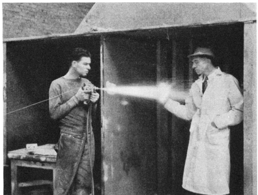
Above: Close-up of the gun that coats anything with metal. Below: Demonstrating the fact that the sprayed metal, a short distance from the spray gun, does not burn
