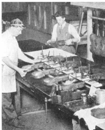
Final assembly of the parts including the fingerboard and bridge
