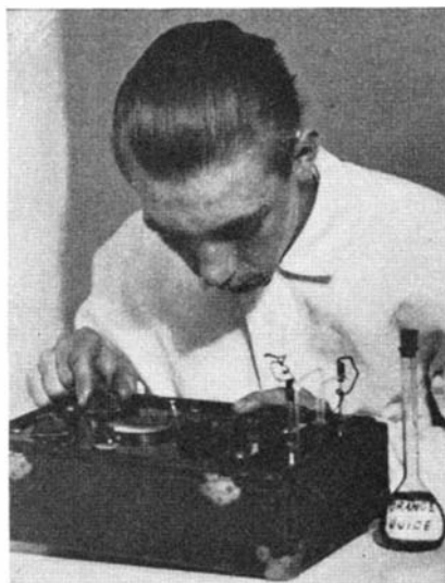
Tester for determining freshness of liquid foods, used in Birdseye laboratory. Electrical resistance of the liquid indicates its freshness
