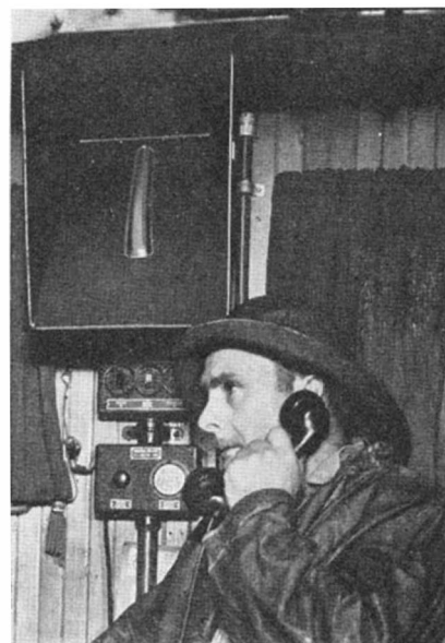
The "telephone booth" on a fishing boat, showing (top) the loudspeaker that replaces the phone bell
