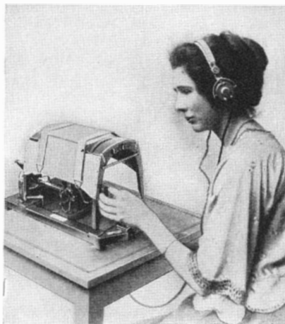
Above: A demonstration of the Optophone with which the blind can read by ear. Left: The pierced disk which "scans" the printed page
