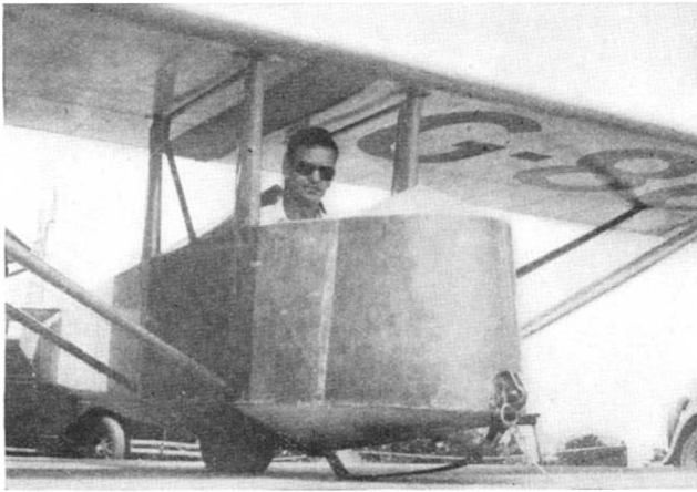
A type of glider for auto-towing in which the pilot is protected by an enclosed cockpit, and by wing structure
