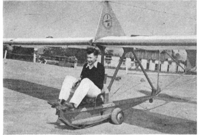
A German training glider. The wheels, slightly behind the center of gravity, help to prevent nose-over tendencies
