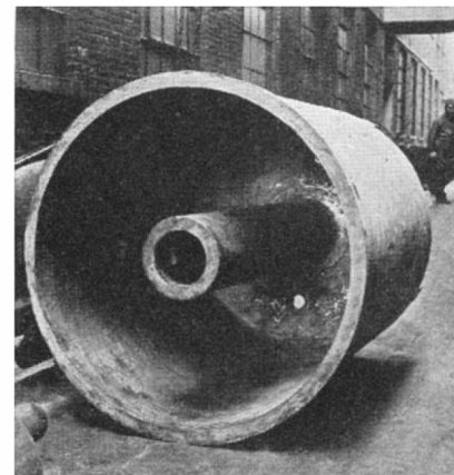
A two-ton carburizing retort made of an alloy of chromium and nickel
