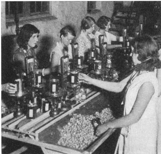
The washed, blanched, and cooked mushrooms are weighed in cans before filling with brine
