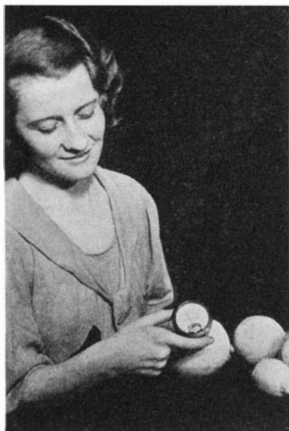
When the two dissimilar pins of this instrument are punched into fruit skins, ripeness is indicated
