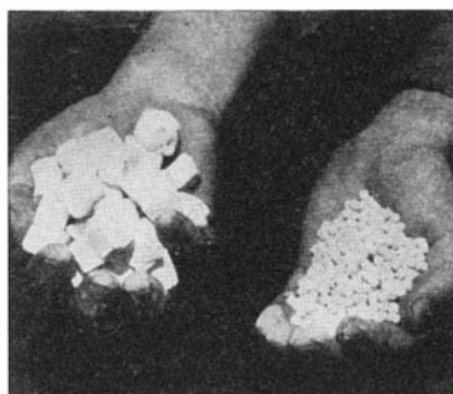
Not pills and lumps of sugar but two forms of the catalyst which boss the high-pressure tower process
