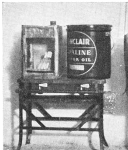
The sterilizers—hot-air (on left) and steam (right) ready for use, on a small gas stove. The motor oil industry contributed both articles
