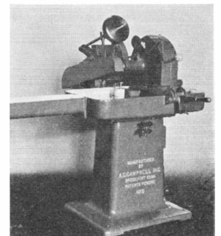
New cutting machine in which the work is kept submerged in a bath
