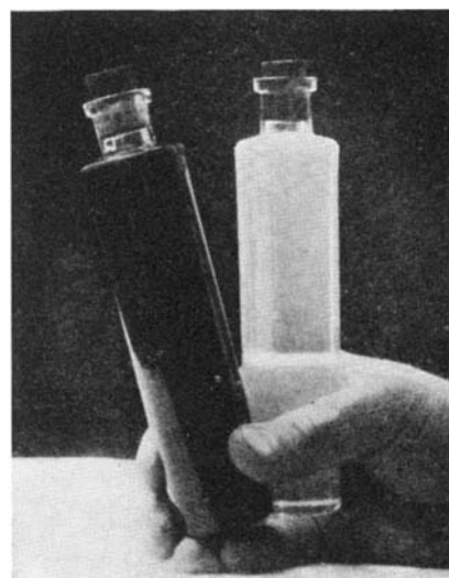
Before and after. A sample of heavy crude oil and a sample of clear, high-octane gasoline it produces
