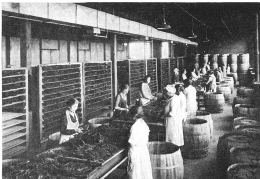
In processing tobacco it is important that the leaves do not dry out and cause dust. Conditioned air, from the overhead duct, “conditions” tobacco here
