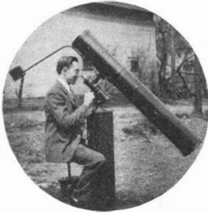
A 6-inch telescope constructed of pipe fittings by Delmar C. Lemmon, instructor in biology in the Roosevelt High School, Dover, Ohio. "I found all the work intensely interesting," Mr. Lemmon writes. "When I return home at evening, tired of working with people all day, I spend many pleasant hours in my basement shop working with things. The total cost of materials was about 50 dollars, and the fun was easily worth twice that much"
