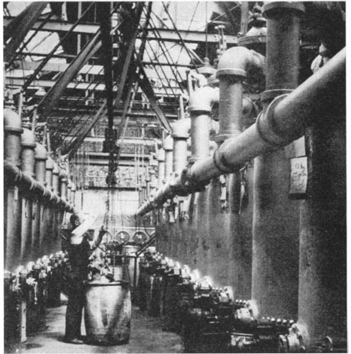
Here the varied elements of the finished coating composition are mixed into one. In the files in this room are formulas for 12,000 colors and shades, all properly classified and indexed. Shadings so subtle that the untrained eye could not identify them are cross-indexed so the key can be found when called for by a manufacturer. A trial batch of the color is made up by hand and is then matched up against the factory mixture which is loaded in great churns or mixers
