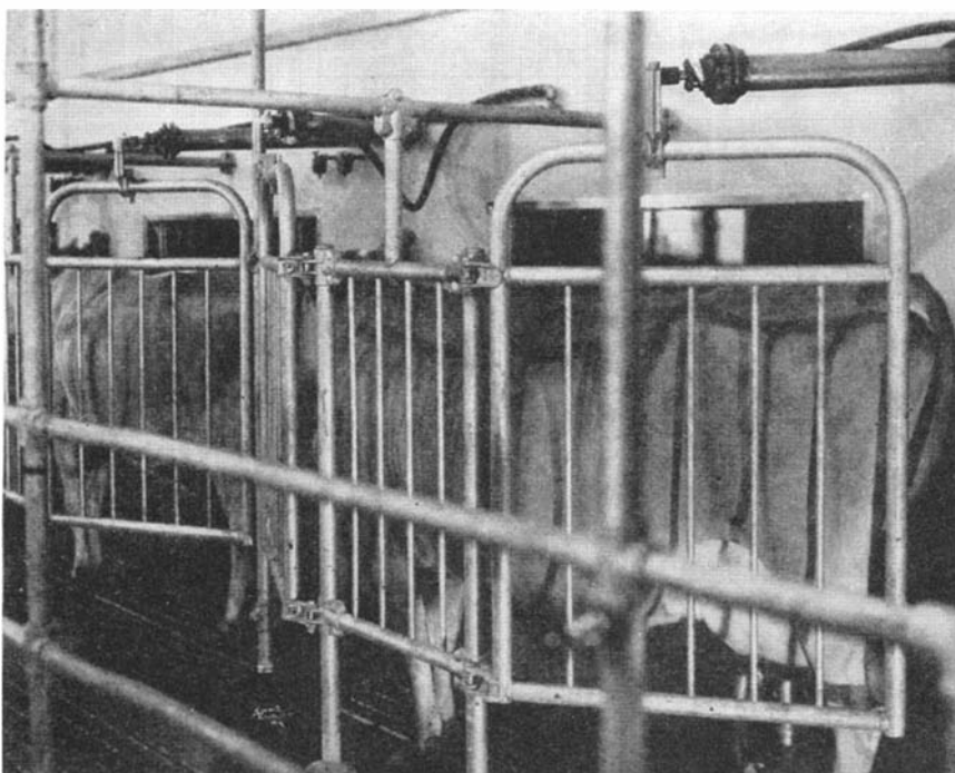
Air gates which regulate the incoming and outgoing of the cows. Each gate is operated by means of compressed air and a piston which is seen at the top
