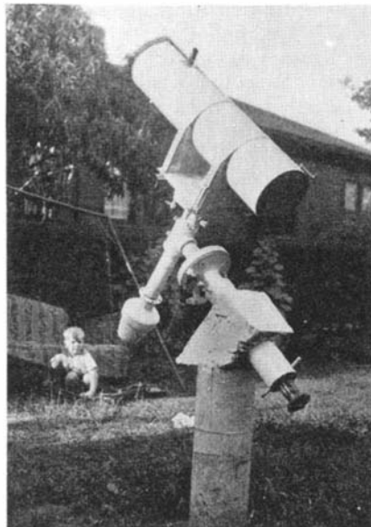
An 8-inch telescope of 32 inches focal length, made by Charles H. Boyd, 3315 Ave. L, Brooklyn, N. Y. He states that he hit on the paraboloidal curve by luck! Some hit on another curve—without luck
