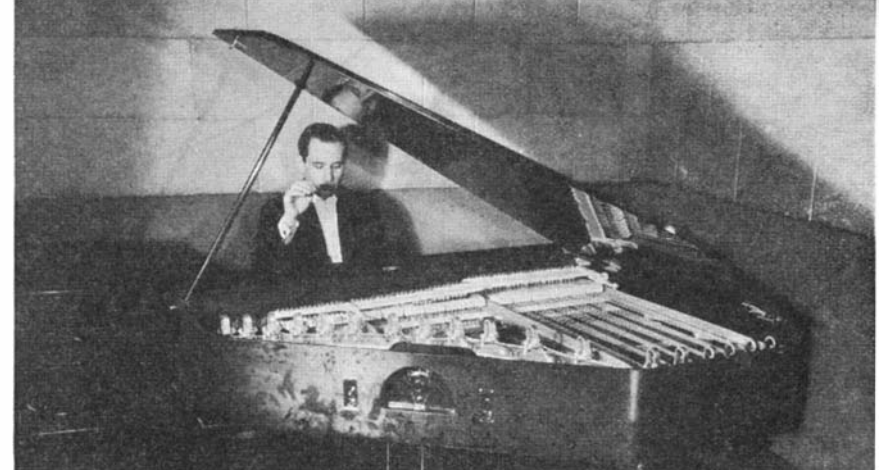
The latest development in pianos. Microphones pick up and amplify the tones
