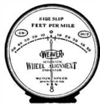
Below: A car rolls upon the wheel-alignment indicator. At left: Sideslip in feet per mile is registered on dial
