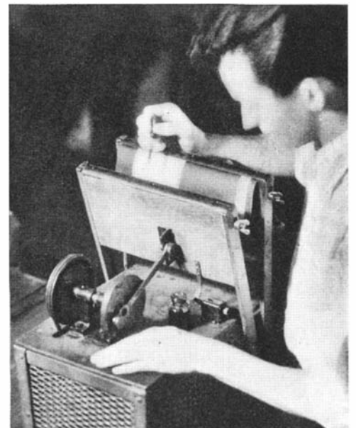
Left: Since Fabrikoid is subject to much scuffing and rubbing when used for book covers, upholstery, cushions, luggage, and so on, the "abrader" tester was developed for making specific tests; it determines the resistance of the coated fabric to abrasion, testing both the film and the color
