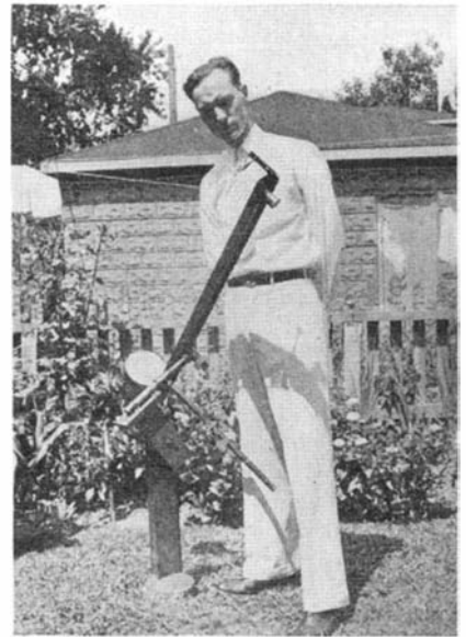
J. H. Nelson, 1036 41st Street, Brooklyn, N. Y., and his 6-inch tubeless telescope. Its "spinal column" is a channel bar of aluminum. This is Mr. Nelson's second telescope and it magnifies 192 diameters. "It took me five months to make my first mirror and 12 hours to complete the second. Even slight experience counts in this hobby," he writes. "I have been badly bitten by the telescope making bug"
