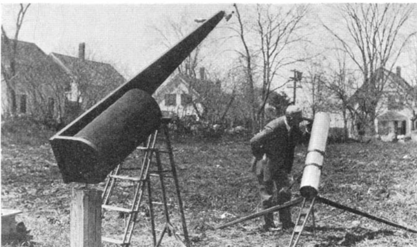
An 8-inch telescope of 32 inches focal length, made by Charles H. Boyd, 3315 Ave. L, Brooklyn, N. Y. He states that he hit on the paraboloidal curve by luck! Some hit on another curve—without luck
