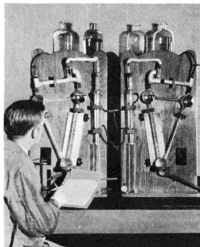
The glass "boilers" for testing the effectiveness of the treatments that may be prescribed for feed-waters
