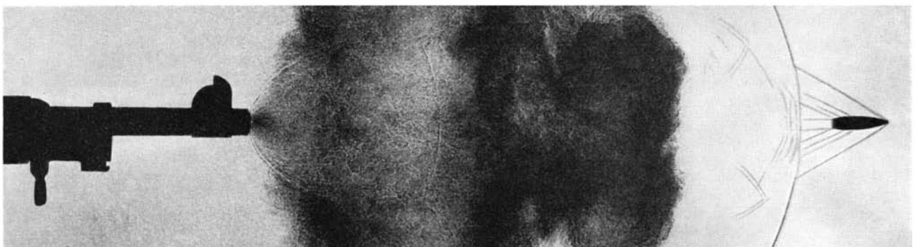
Right: Leakage gas from shot shell with inferior wadding. Below: Bullet, propelling gas, and sound waves from .30 caliber Springfield. See text, above at right
