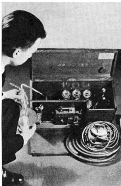
A compact kit for collecting certain dusts and vapors from the air
