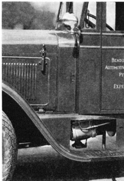
The air steering control unit, an aluminum cylinder, under chassis
