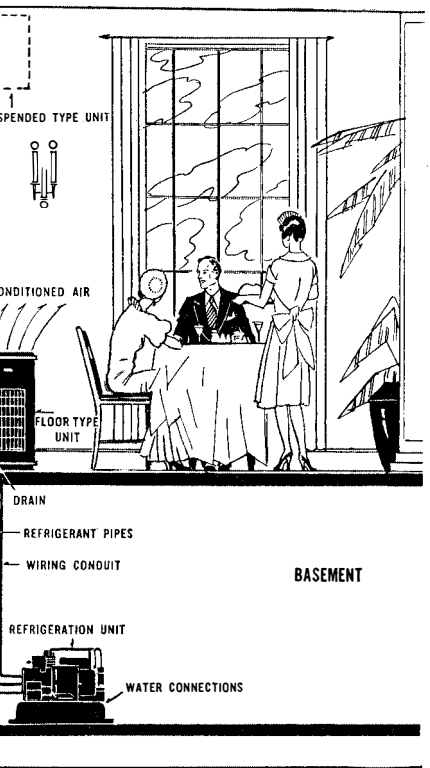
Typical air-conditioning installation with the refrigerating equipment in the basement
