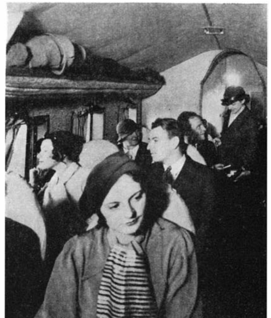
In the cabin of a Condor, showing the sound-absorbing fabric on the walls and ceiling
