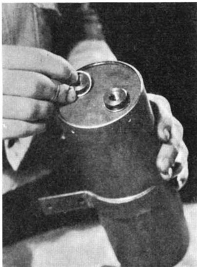
Preparation for welding requires a snug fit of parts and application of copper or copper paste at or near joint. Below: A large number of welds may be made at one time
