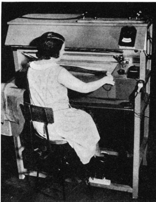
Grading hosiery for evenness in a grading cabinet, with measured light and light filters
