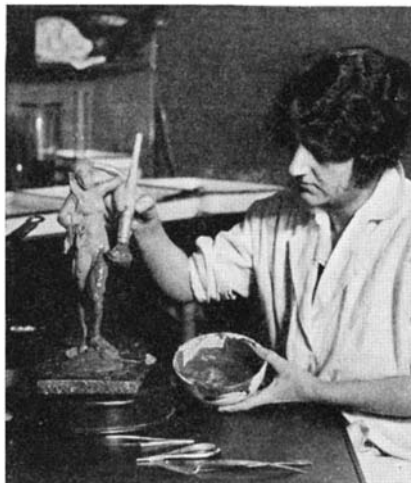
The first step in the new moulage process: applying the Negocoll to a small statuette by means of a brush
