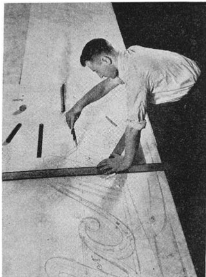
Making the pattern from which a gaseous tube sign will be laid out
