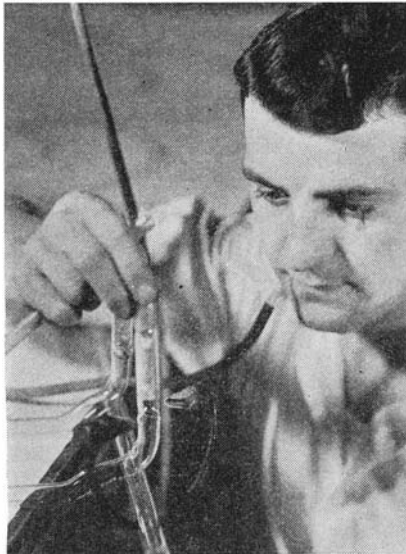
The short glass tube (see photo at left) is sealed to a glass sign tube
