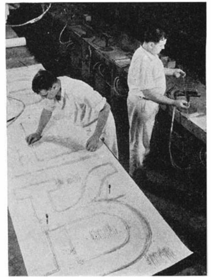
Bending sign tubes to shape on a full-size pattern drawn on asbestos
