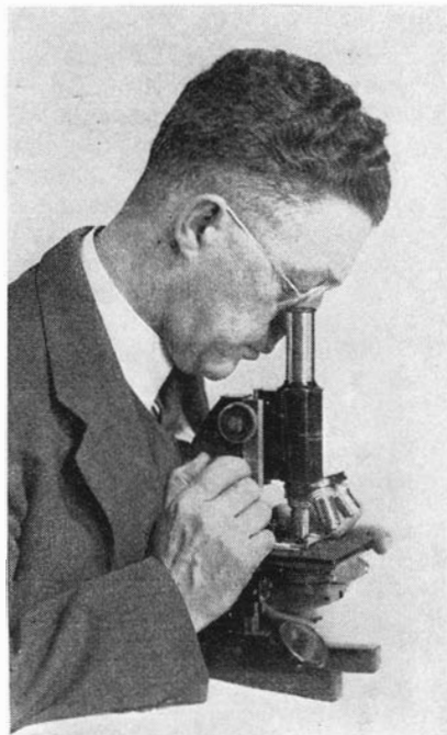
How the right hand is rested on the stage for the easy manipulation of the fine adjustments. It gives accurate and steady control
