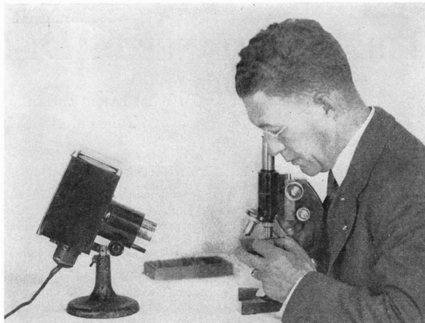
Showing the correct method of bracing the left hand when moving the slide: thumb and forefinger are grasping the slide, the middle finger on the stage
