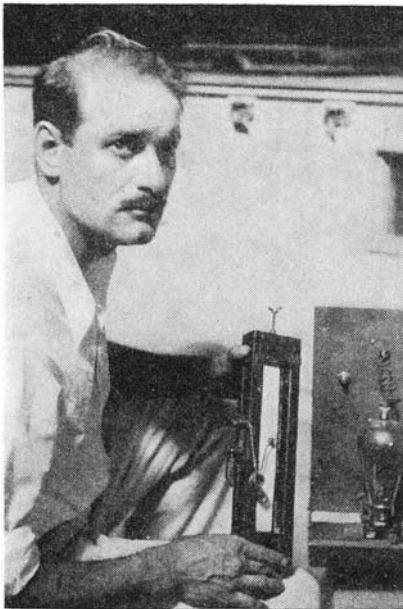
The wood hygrostat with contacts to operate a vacuum tube circuit
