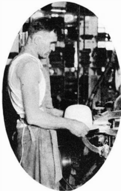
Coated abrasives used in finishing a felt hat. At left: Small and large rotating implements use sandpaper
