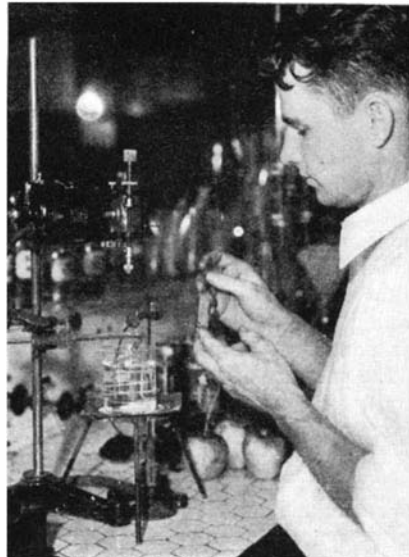
A near view of the electrolytic apparatus for lead determination
