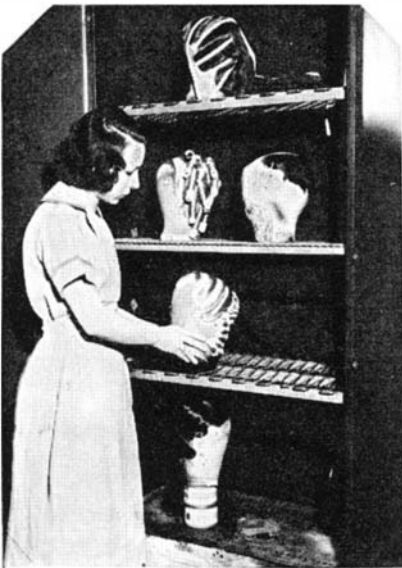
After a wig is completed and waved as desired, it is baked in an oven for four hours at 110 degrees to "set" the wave
