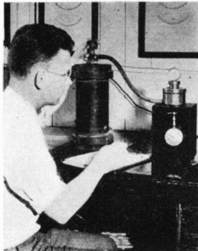
Drainage indicator, used in road building research, shows rise of water in soil sample under pressure
