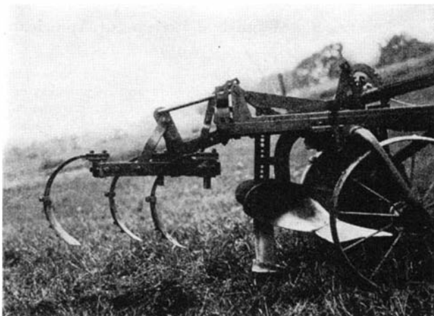
Two views of the reforestation plow. At left are shown sod cutter, sub-soiler, and cultivator teeth. Plow in use at right
