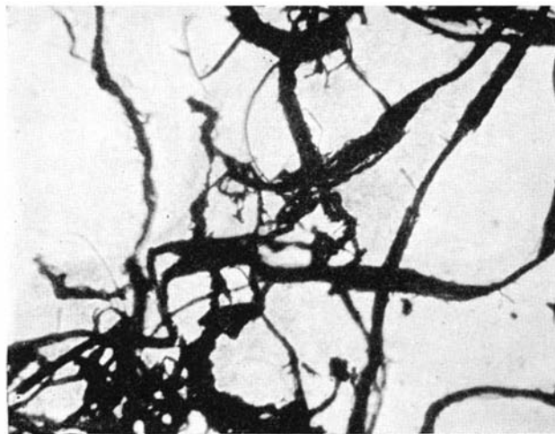
Photomicrographs showing above: Excellent shape for sandpaper grains for strength and sharpness; and below: Wood shavings, not dust, are cut by sandpaper
