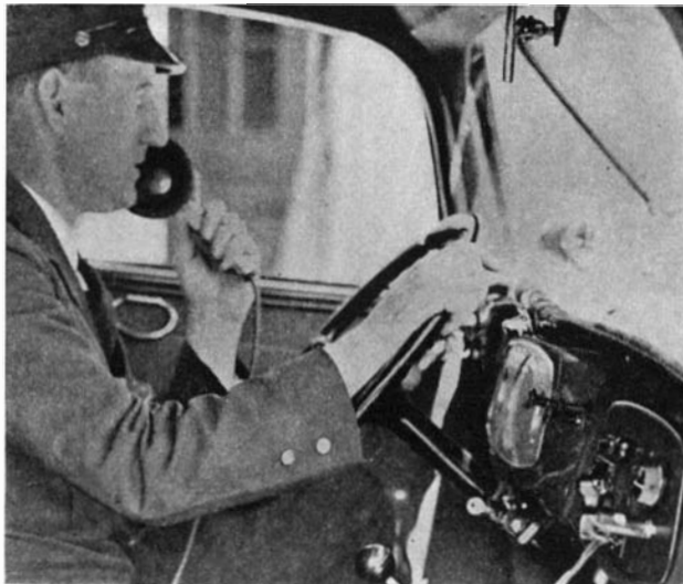
Interior of two-way radio police cruiser, with equipment built into the instrument panel of the car
