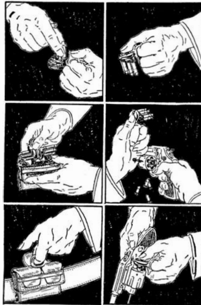
The new revolver cartridge clip. Read left column down, then right
