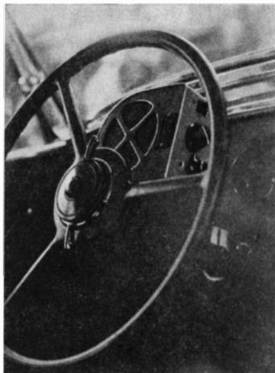
Steering-column type equipment, showing the small dynamic speaker
